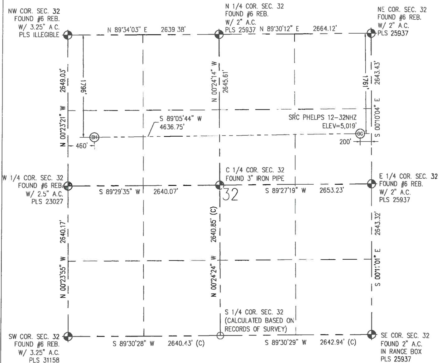
IN ACCORDANCE WITH A REQUEST FROM CRAIG RASMUSON - SYNERGY RESOURCES, BASELINE ENGINEERING CORP. HAS DETERMINED THE LOCATION OF THE SRC PHELPS 12-32NHZ AND 200' FEL, AS MEASURED AT NINETY (90) DEGREES FROM THE SECTION LINE OF SECTION 32, TOWNSHIP 1 NORTH, RANGE 66 WEST AND THE BOTTOM HOLE LOCATION TO BE 1,796' FNL AND 460' FW. OF SECTION 32, TOWNSHIP 1 NORTH, RANGE 66 WEST, 6TH PRINCIPAL MERIDIAN, WELD COUNTY, COLORADO.
