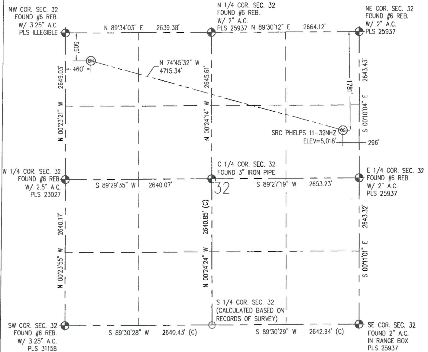
IN ACCORDANCE WITH A REQUEST FROM CRAIG RASMUSON - SYNERGY RESOURCES, BASELINE ENGINEERING CORP. HAS DETERMINED THE LOCATION OF THE SRC PHELPS 11-32NHZ TO BE 1,781' FNL AND 296' FEL, AS MEASURED AT NINETY (90) DEGREES FROM THE SECTION LINE OF SECTION 32, TOWNSHIP 1 NORTH, RANGE 66 WEST AND THE BOTTOM HOLE LOCATION TO BE 505' FNL AND 460' FWL OF SECTION 32, TOWNSHIP 1 NORTH, RANGE 66 WEST, 6TH PRINCIPAL MERIDIAN, WELD COUNTY, COLORADO
