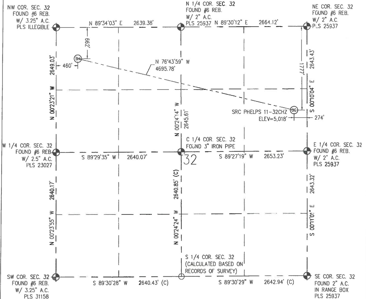
IN ACCORDANCE WITH A REQUEST FROM CRAIG RASMUSON - SYNERGY RESOURCES, BASELINE ENGINEERING CORP. HAS DETERMINED THE LOCATION OF THE SRC PHELPS 11-32CHZ TO BE 1,777' FNL AND 274' FEL, AS MEASURED AT NINETY (90) DEGREES FROM THE SECTION LINE OF SECTION 32, TOWNSHIP 1 NORTH, RANGE 66 WEST AND THE BOTTOM HOLE LOCATION TO BE 662' FNL AND 460' FEL OF SECTION 32, TOWNSHIP 1 NORTH, RANGE 66 WEST, 6TH PRINCIPAL MERIDIAN, WELD COUNTY, COLORADO.
