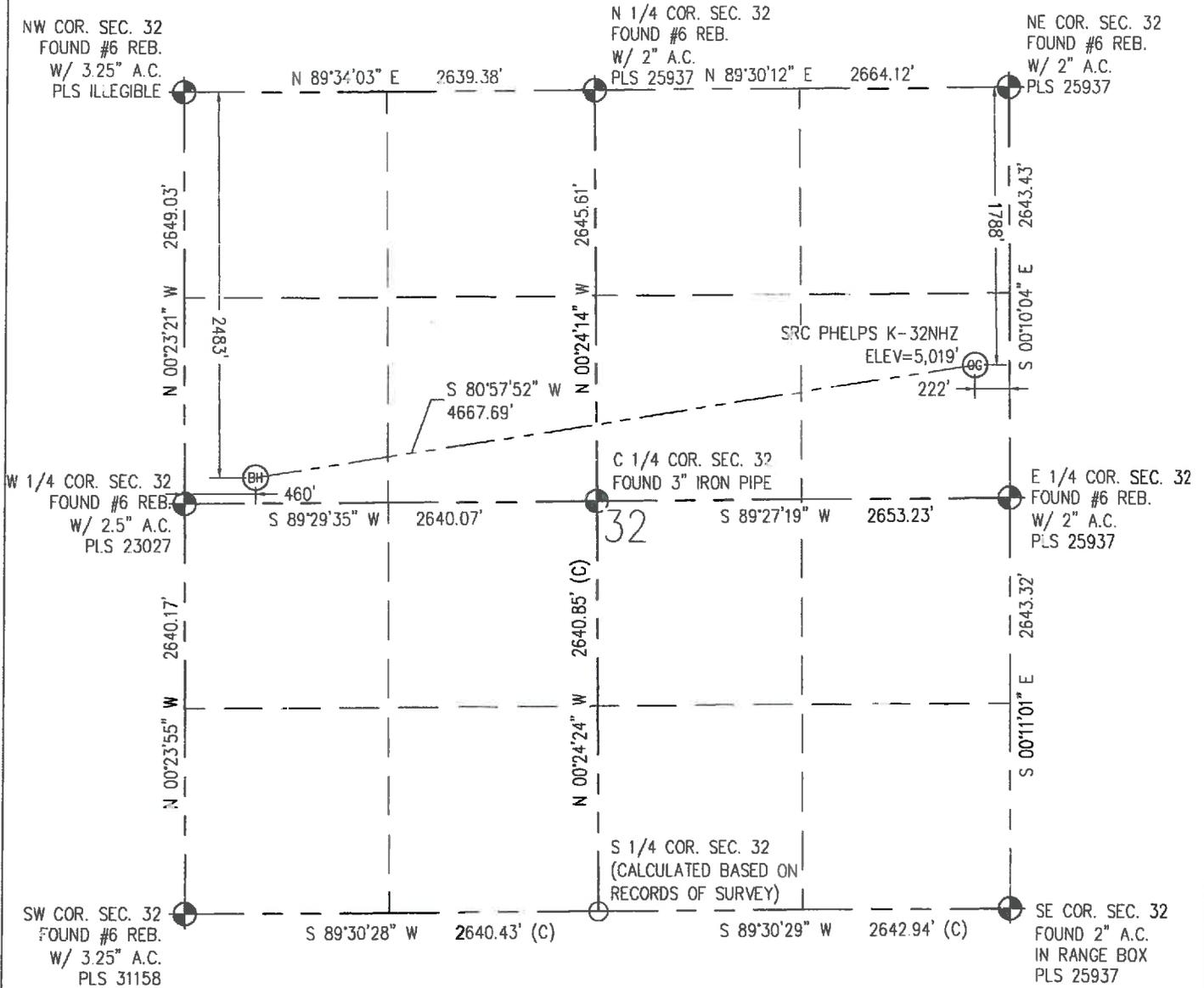
IN ACCORDANCE WITH A REQUEST FROM CRAIG RASMUSON - SYNERGY RESOURCES, BASELINE ENGINEERING CORP. HAS DETERMINED THE LOCATION OF THE SRC PHELPS K-32NHZ TO BE 1,788' FNL AND 222' FEL, AS MEASURED AT NINETY (90) DEGREES FROM THE SECTION LINE OF SECTION 32, TOWNSHIP 1 NORTH, RANGE 66 WEST AND THE BOTTOM HOLE LOCATION TO BE 2,483' FNL AND 460' FNL OF SECTION 32, TOWNSHIP 1 NORTH, RANGE 66 WEST, 6TH PRINCIPAL MERIDIAN, WELD COUNTY, COLORADO.
