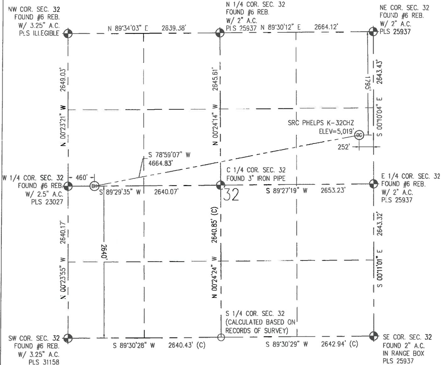
IN ACCORDANCE WITH A REQUEST FROM CRAIG RASMUSON - SYNERGY RESOURCES, BASELINE ENGINEERING CORP. HAS DETERMINED THE LOCATION OF THE SRC PHELPS K-32CHZ TO BE 1,795' FNL AND 252' FEL, AS MEASURED AT NINETY (90) DEGREES FROM THE SECTION LINE OF SECTION 32, TOWNSHIP 1 NORTH, RANGE 66 WEST, AND THE BOTTOM HOLE LOCATION TO BE 2,640' FSL AND 460' FWL OF SECTION 32, TOWNSHIP 1 NORTH, RANGE 66 WEST, 6TH PRINCIPAL MERIDIAN, WELD COUNTY, COLORADO.
