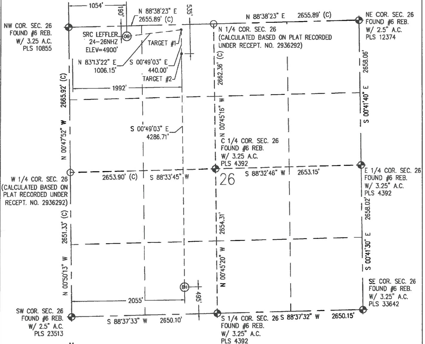
IN ACCORDANCE WITH A REQUEST FROM CRAIG RASMUSON - SYNERGY RESOURCES, BASELINE ENGINEERING CORP. HAS DETERMINED THE LOCATION OF THE SRC LEFFLER 24-26NHZ TO BE 190' FNL AND 1054' FNL, AS MEASURED AT NINETY (90) DEGREES FROM THE SECTION LINE OF SECTION 26, TOWNSHIP 7 NORTH, RANGE 66 WEST AND THE BOTTOM HOLE LOCATION TO BE 495' FSL AND 2055' FNL OF SECTION 26, TOWNSHIP 7 NORTH, RANGE 66 WEST, 6TH PRINCIPAL MERIDIAN, WELD COUNTY, COLORADO.
