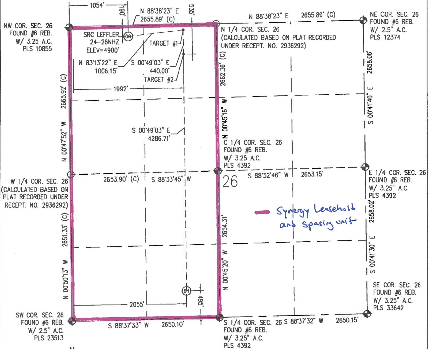
IN ACCORDANCE WITH A REQUEST FROM CRAIG RASMUSON - SYNERGY RESOURCES, BASELINE ENGINEERING CORP. HAS DETERMINED THE LOCATION OF THE SRC LEFFLER 24-26NHZ TO BE 190' FNL AND 1054' FWL, AS MEASURED AT NINETY (90) DEGREES FROM THE SECTION LINE OF SECTION 26, TOWNSHIP 7 NORTH, RANGE 66 WEST AND THE BOTTOM HOLE LOCATION TO BE 495' FSL AND 2055' FWL OF SECTION 26, TOWNSHIP 7 NORTH, RANGE 66 WEST, 6TH PRINCIPAL MERIDIAN, WELD COUNTY, COLORADO.
