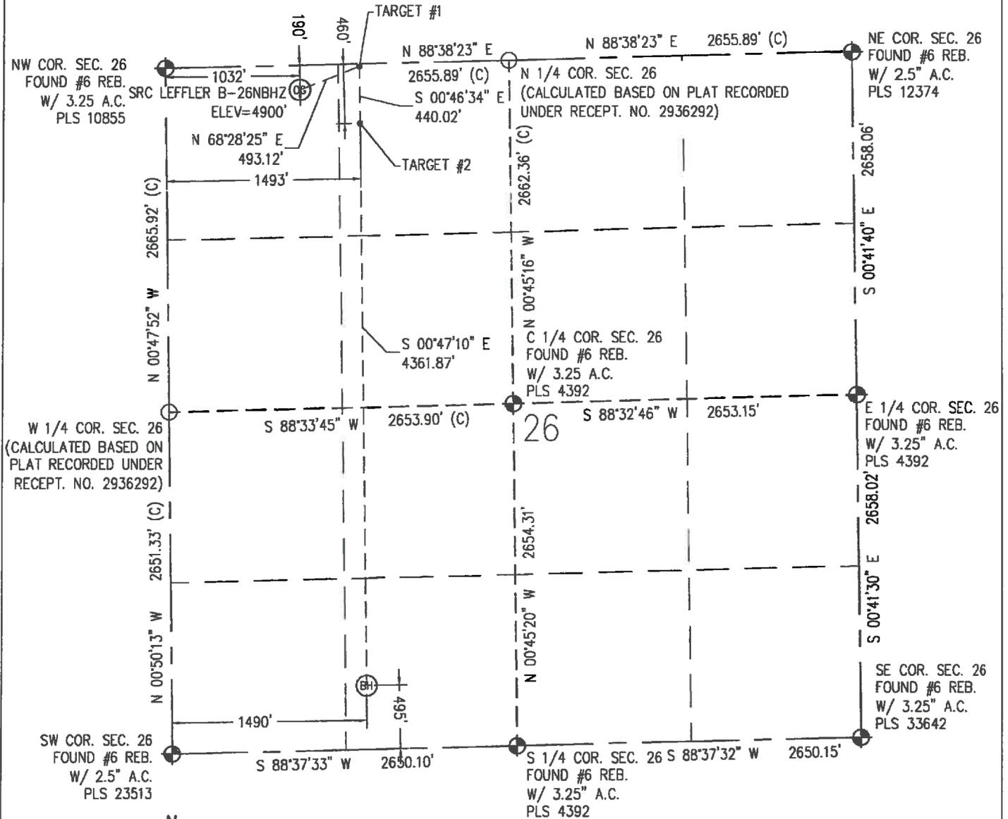
IN ACCORDANCE WITH A REQUEST FROM CRAIG RASMUSON - SYNERGY RESOURCES, BASELINE ENGINEERING CORP. HAS DETERMINED THE LOCATION OF THE SRC LEFFLER B-26NBHZ TO BE 190' FNL AND 1032' FWL, AS MEASURED AT NINETY (90) DEGREES FROM THE SECTION LINE OF SECTION 26, TOWNSHIP 7 NORTH, RANGE 66 WEST AND THE BOTTOM HOLE LOCATION TO BE 495' FSL AND 1490' FWL OF SECTION 26, TOWNSHIP 7 NORTH, RANGE 66 WEST, 6TH PRINCIPAL MERIDIAN, WELD COUNTY, COLORADO.
