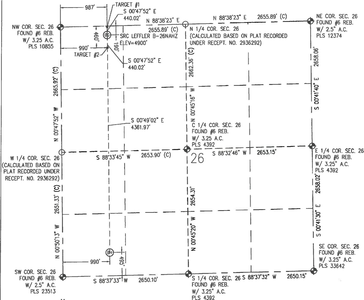
IN ACCORDANCE WITH A REQUEST FROM CRAIG RASMUSON - SYNERGY RESOURCES, BASELINE ENGINEERING CORP. HAS DETERMINED THE LOCATION OF THE SRC LEFFLER B-26NAHZ TO BE 190' FNL AND 987' FWL, AS MEASURED AT NINETY (90) DEGREES FROM THE SECTION LINE OF SECTION 26, TOWNSHIP 7 NORTH, RANGE 66 WEST AND THE BOTTOM HOLE LOCATION TO BE 495' FSL AND 990' FWL OF SECTION 26, TOWNSHIP 7 NORTH, RANGE 66 WEST, 6TH PRINCIPAL MERIDIAN, WELD COUNTY, COLORADO.
