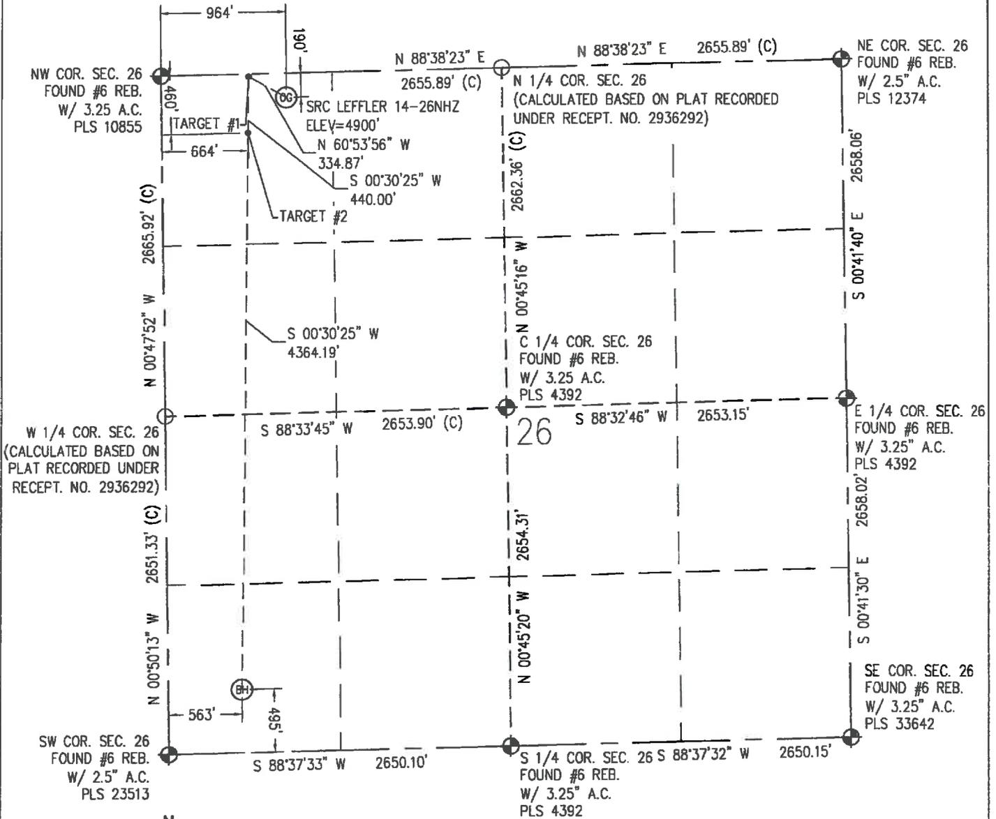
IN ACCORDANCE WITH A REQUEST FROM CRAIG RASMUSON - SYNERGY RESOURCES, BASELINE ENGINEERING CORP. HAS DETERMINED THE LOCATION OF THE SRC LEFFLER 14-26NHZ TO BE 190' FNL AND 964' FWL, AS MEASURED AT NINETY (90) DEGREES FROM THE SECTION LINE OF SECTION 26, TOWNSHIP 7 NORTH, RANGE 66 WEST AND THE BOTTOM HOLE LOCATION TO BE 495' FSL AND 563' FWL OF SECTION 26, TOWNSHIP 7 NORTH, RANGE 66 WEST, 6TH PRINCIPAL MERIDIAN, WELD COUNTY, COLORADO.
