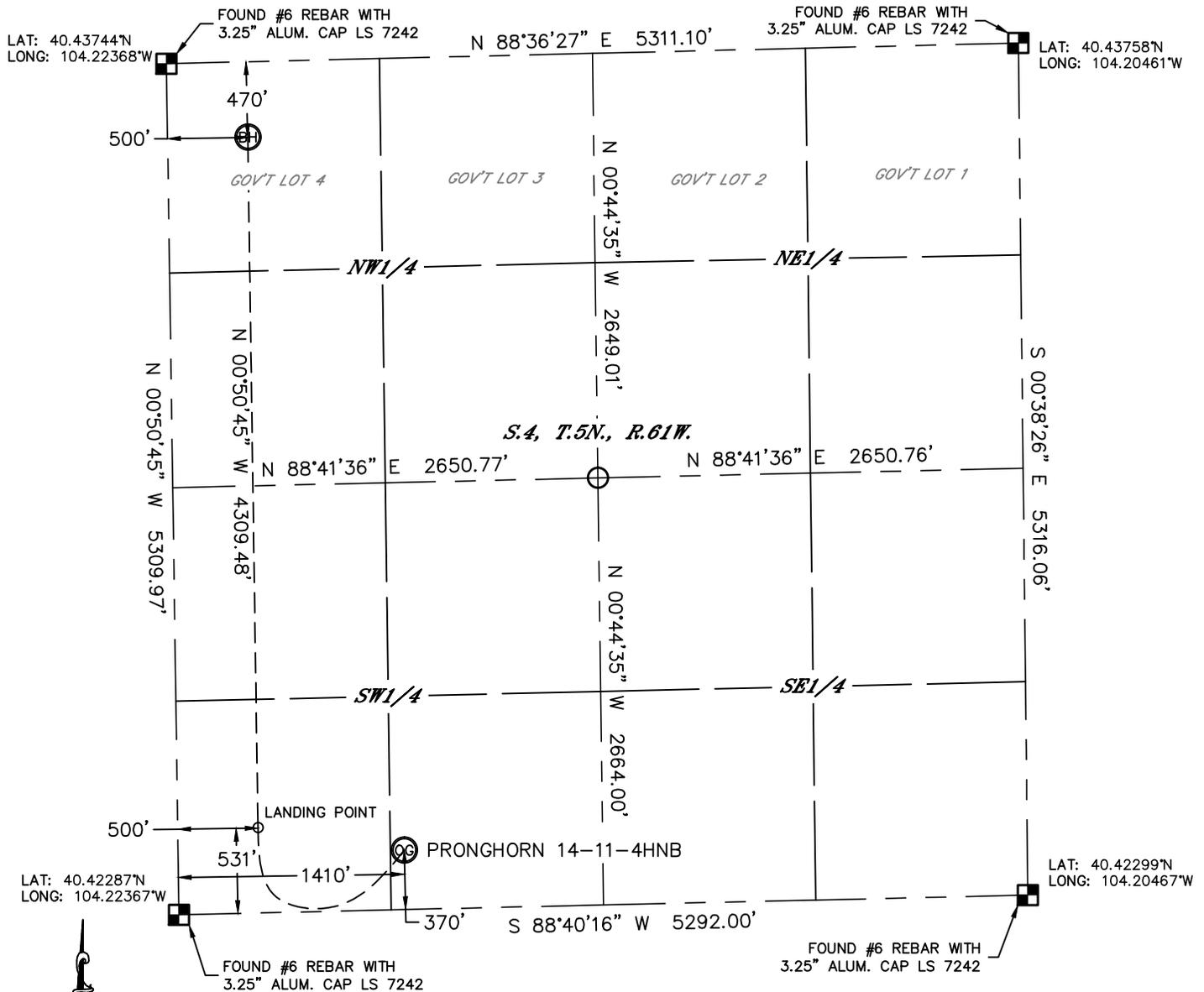
In accordance with a request from Michael Meagher with BONANZA CREEK ENERGY, INC. Lat40°, Inc. has determined the surface location of the PRONGHORN 14-11-4HNB to be 370' from the SOUTH line and 1410' from the WEST line and the bottom hole to be 470' from the NORTH line and 500' from the WEST line as measured at right angles from the section lines of Section 4, Township 5 North, Range 61 West of the Sixth Principal Meridian, County of Weld, State of Colorado.
