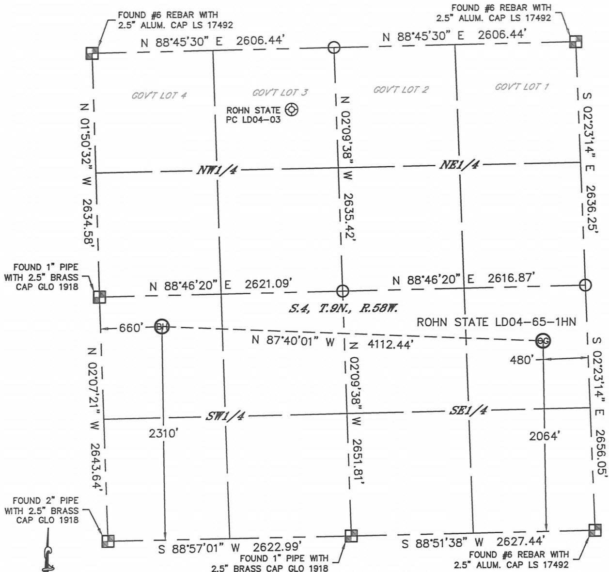
In accordance with a request from Nate McCorkell with Noble Energy Inc., Lat40°, Inc. has determined the surface location of the ROHN STATE LD04-65-1HN to be 2064' from the SOUTH line and 480' from the EAST line and the bottom hole to be 2310' from the SOUTH line and 660' from the WEST line as measured at right angles from the section lines of Section 4, Township 9 North, Range 58 West of the Sixth Principal Meridian, County of Weld, State of Colorado.
