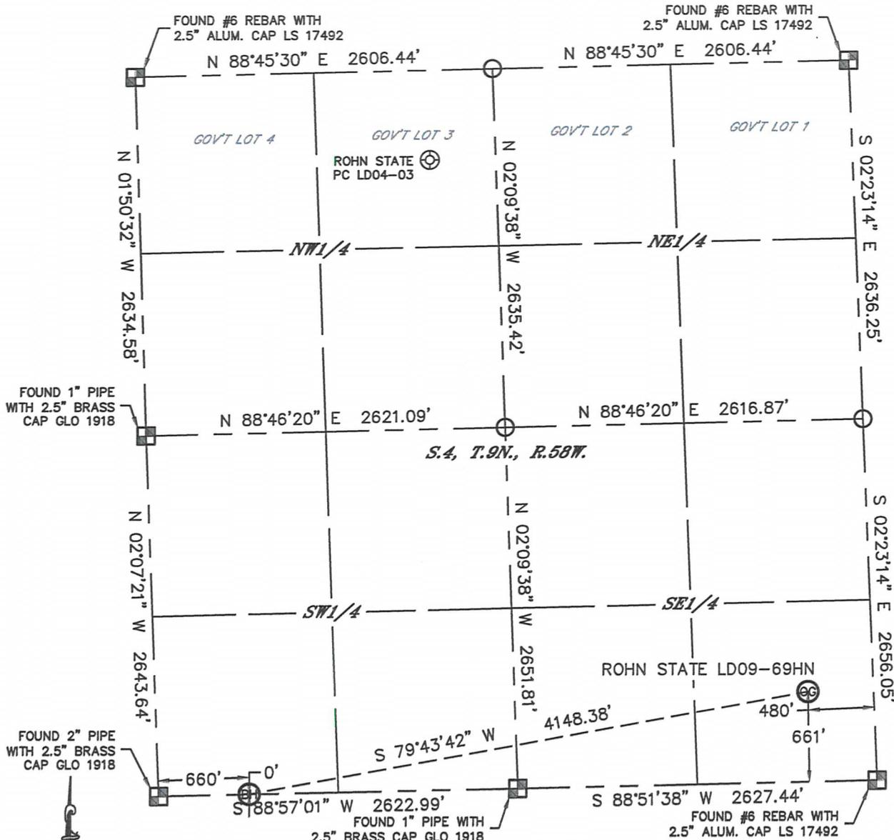
In accordance with a request from Nate McCorkell with Noble Energy Inc. Lat40°, Inc. has determined the surface location of the ROHN STATE LD09-69HN to be 661' from the SOUTH line and 480' from the EAST line and the bottom hole to be 0' from the SOUTH line and 660' from the WEST line as measured at right angles from the section lines of Section 4, Township 9 North, Range 58 West of the Sixth Principal Meridian, County of Weld, State of Colorado.
