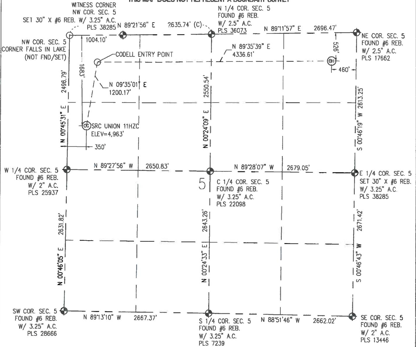
IN ACCORDANCE WITH A REQUEST FROM CRAIG RASMJON - SYNERGY RESOURCES, BASELINE ENGINEERING CORP. HAS DETERMINED THE LOCATION OF THE SRC UNION 11HZC TO BE 1683' FNL AND 350' FWL, AS MEASURED AT NINETY (90) DEGREES FROM THE SECTION LINE OF SECTION 5, TOWNSHIP 2 NORTH, RANGE 68 WEST AND THE BOTTOM HOLE LOCATION TO BE 526' FNL AND 460' FEL OF SECTION 5, TOWNSHIP 2 NORTH, RANGE 68 WEST, 6TH PRINCIPAL MERIDIAN, WELD COUNTY, COLORADO.
