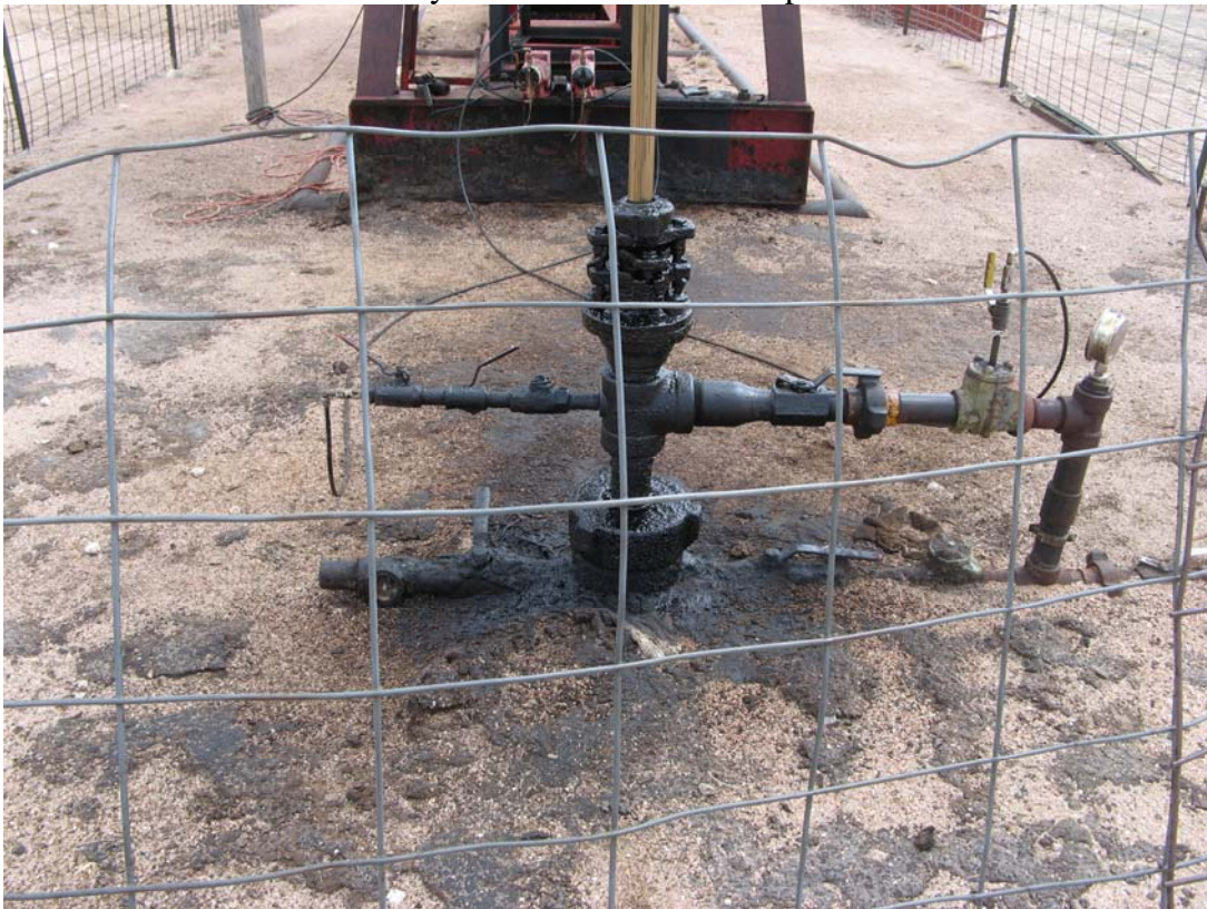
Wellhead – oily waste, leaks
