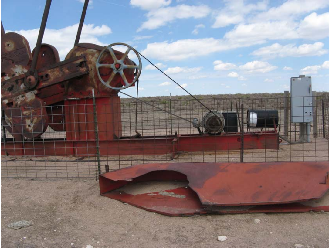
Pumping unit – unprotected belt drive.
