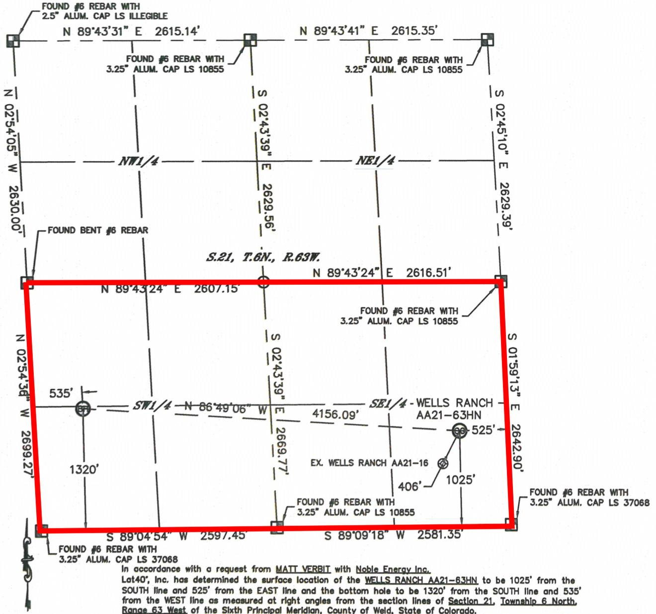
In accordance with a request from MATT VERBIT with Noble Energy Inc. Lat40°, Inc. has determined the surface location of the WELLS RANCH AA21-63HN to be 1025' from the SOUTH line and 525' from the EAST line and the bottom hole to be 1320' from the SOUTH line and 535' from the WEST line as measured at right angles from the section lines of Section 21, Township 6 North, Range 63 West of the Sixth Principal Meridian, County of Weld, State of Colorado.
