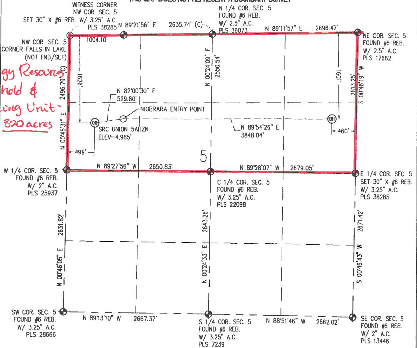
IN ACCORDANCE WITH A REQUEST FROM CRAIG RASMUSON - SYNERGY RESOURCES, BASELINE ENGINEERING CORP. HAS DETERMINED THE LOCATION OF THE SRC UNION 5AHZN TO BE 1626' FNL AND 499' FWL, AS MEASURED AT NINETY (90) DEGREES FROM THE SECTION LINE OF SECTION 5, TOWNSHIP 2 NORTH, RANGE 68 WEST AND THE BOTTOM HOLE LOCATION TO BE 1601' FNL AND 460' FEL OF SECTION 5, TOWNSHIP 2 NORTH, RANGE 68 WEST, 6TH PRINCIPAL MERIDIAN, WELD COUNTY, COLORADO.
