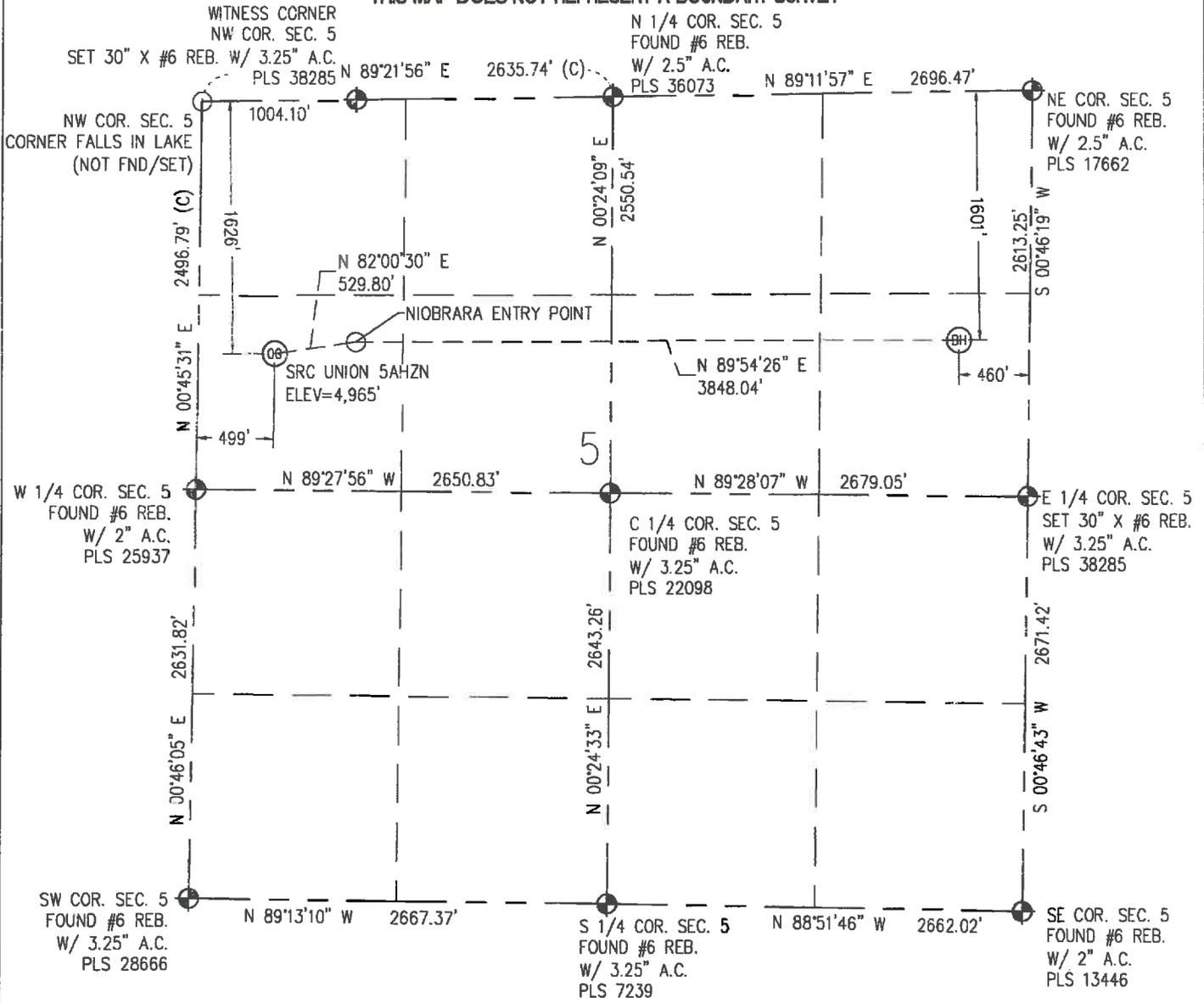
IN ACCORDANCE WITH A REQUEST FROM CRAIG RASMUSON - SYNERGY RESOURCES, BASELINE ENGINEERING CORP. HAS DETERMINED THE LOCATION OF THE SRC UNION SAHZN TO BE 1626' FNL AND 499' FWL, AS MEASURED AT NINETY (90) DEGREES FROM THE SECTION LINE OF SECTION 5, TOWNSHIP 2 NORTH, RANGE 68 WEST AND THE BOTTOM HOLE LOCATION TO BE 1601' FNL AND 460' FEL OF SECTION 5, TOWNSHIP 2 NORTH, RANGE 68 WEST, 6TH PRINCIPAL MERIDIAN, WELD COUNTY, COLORADO.
