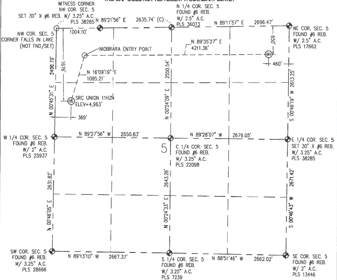
IN ACCORDANCE WITH A REQUEST FROM CRAIG RASMUSON - SYNERGY RESOURCES, BASELINE ENGINEERING CORP HAS DETERMINED THE LOCATION OF THE SRC UNION 11HZN TO BE 1676' FNL AND 369' FWL, AS MEASURED AT NINETY (90) DEGREES FROM THE SECTION LINE OF SECTION 5, TOWNSHIP 2 NORTH, RANGE 68 WEST AND THE BOTTOM HOLE LOCATION TO BE 650' FNL AND 460' FEL OF SECTION 5, TOWNSHIP 2 NORTH, RANGE 68 WEST, 6TH PRINCIPAL MERIDIAN, WELD COUNTY, COLORADO.
