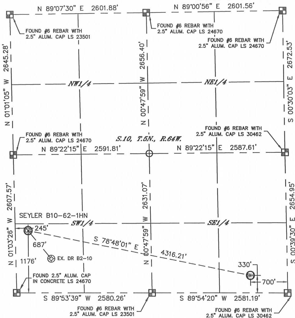
In accordance with a request from Jacob Rice with Noble Energy Inc., Lat40°, Inc. has determined the surface location of the SEYLER B10-62-1HN to be 1176' from the SOUTH line and 245' from the WEST line and the bottom hole to be 330' from the SOUTH line and 700' from the EAST line as measured at right angles from the section lines of Section 10, Township 5 North, Range 64 West of the Sixth Principal Meridian, County of Weld, State of Colorado.
