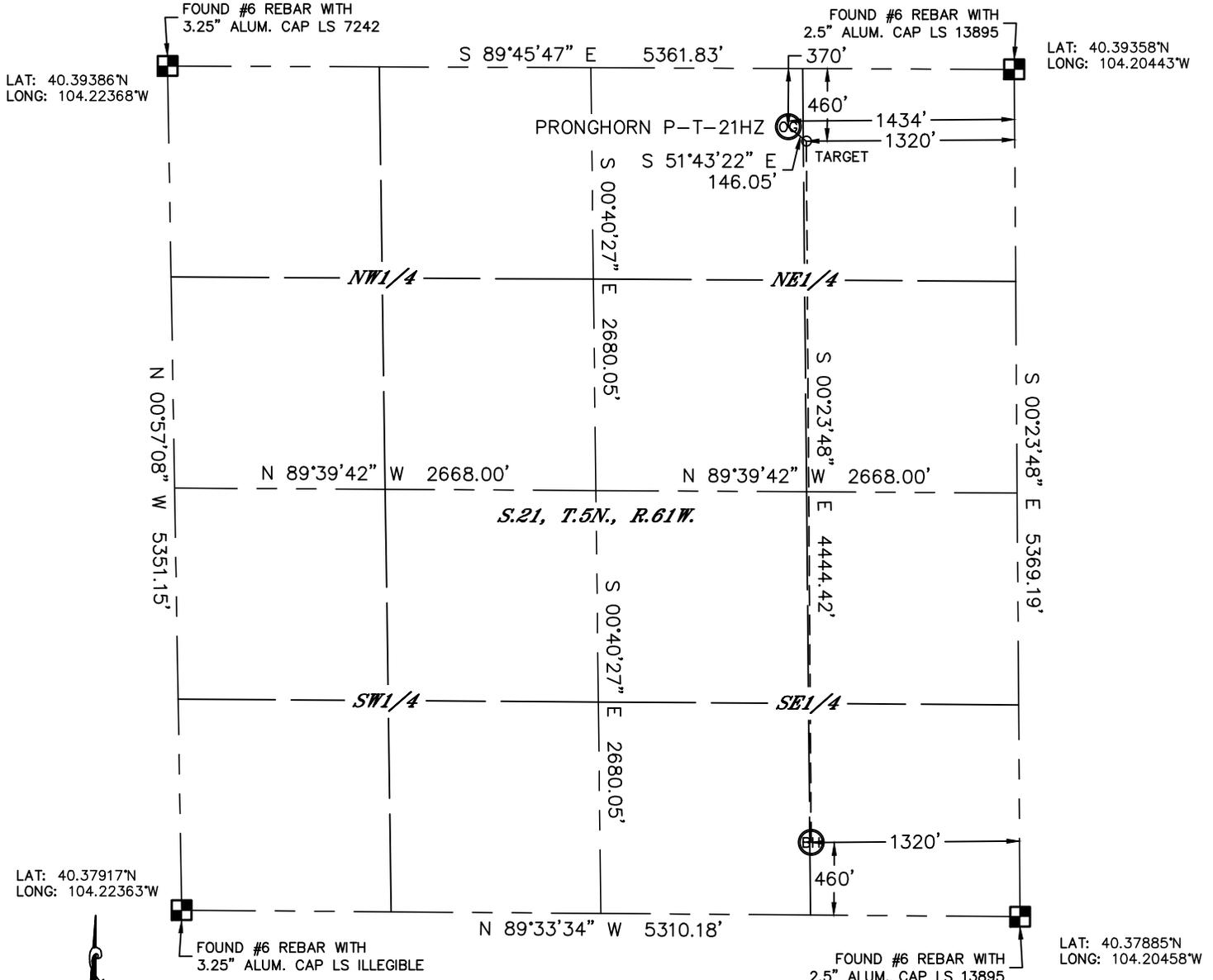
In accordance with a request from Michael Meagher with BONANZA CREEK ENERGY, INC. Lat40°, Inc. has determined the surface location of the PRONGHORN P-T-21HZ to be 370' from the NORTH line and 1434' from the EAST line and the bottom hole to be 460' from the SOUTH line and 1320' from the EAST line as measured at right angles from the section lines of Section 21, Township 5 North, Range 61 West of the Sixth Principal Meridian, County of Weld, State of Colorado.
