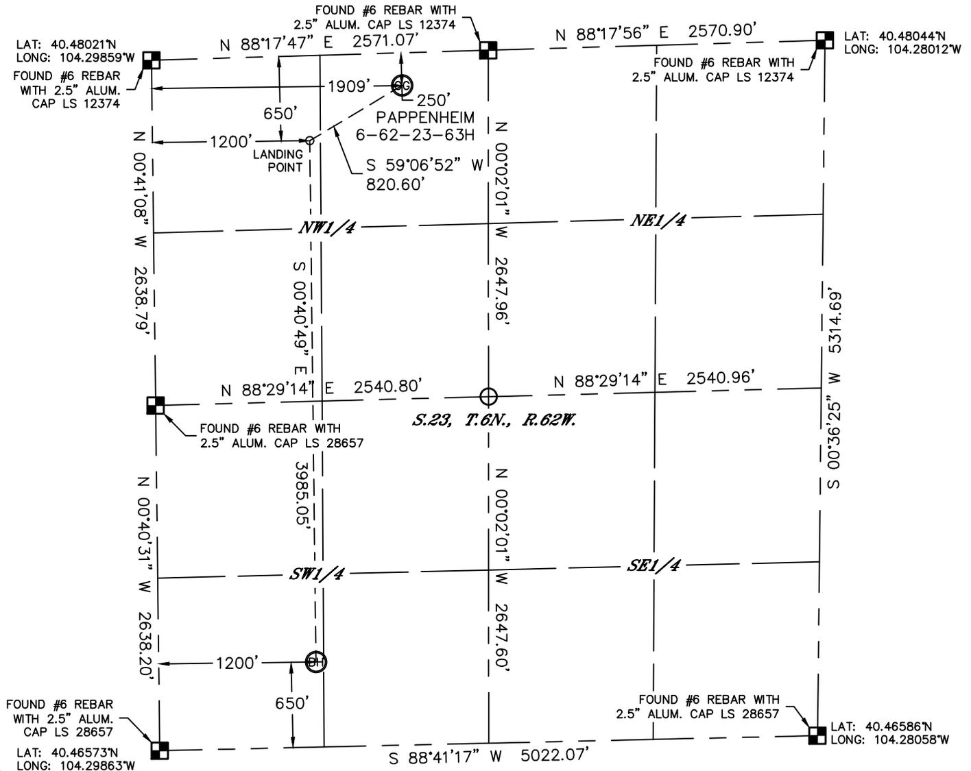
In accordance with a request from Jeff Fandrich with BILL BARRETT CORPORATION Lat40°, Inc. has determined the surface location of the PAPPENHEIM 6-62-23-63H to be 250' from the NORTH line and 1909' from the WEST line and the bottom hole to be 650' from the SOUTH line and 1200' from the WEST line as measured at right angles from the section lines of Section 23, Township 6 North, Range 62 West of the Sixth Principal Meridian, County of Weld, State of Colorado.
