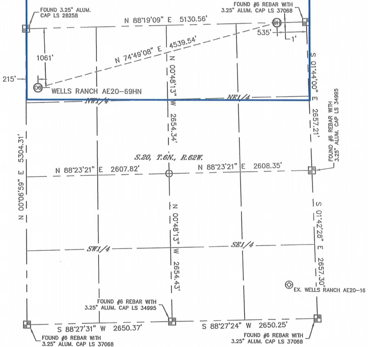
In accordance with a request from Brian James with Noble Energy Inc., Lat40, Inc. has determined the surface location of the WELLS RANCH AE20-69HN to be 1061' from the NORTH line and 215' from the WEST line and the bottom hole to be 1' from the NORTH line and 535' from the EAST line as measured at right angles from the section lines of Section 20, Township 6 North, Range 62 West of the Sixth Principal Meridian, County of Weld, State of Colorado.
