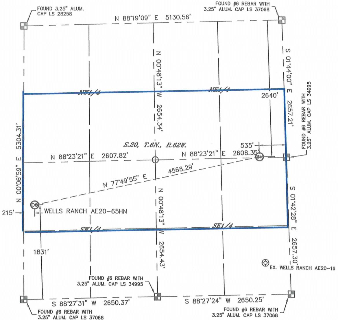
In accordance with a request from Brian James with Noble Energy Inc. Lat40°, Inc. has determined the surface location of the WELLS RANCH AE20-65HN to be 1831' from the SOUTH line and 215' from the WEST line and the bottom hole to be 2640' from the NORTH line and 535' from the EAST line as measured at right angles from the section lines of Section 20, Township 6 North, Range 62 West of the Sixth Principal Meridian, County of Weld, State of Colorado.
