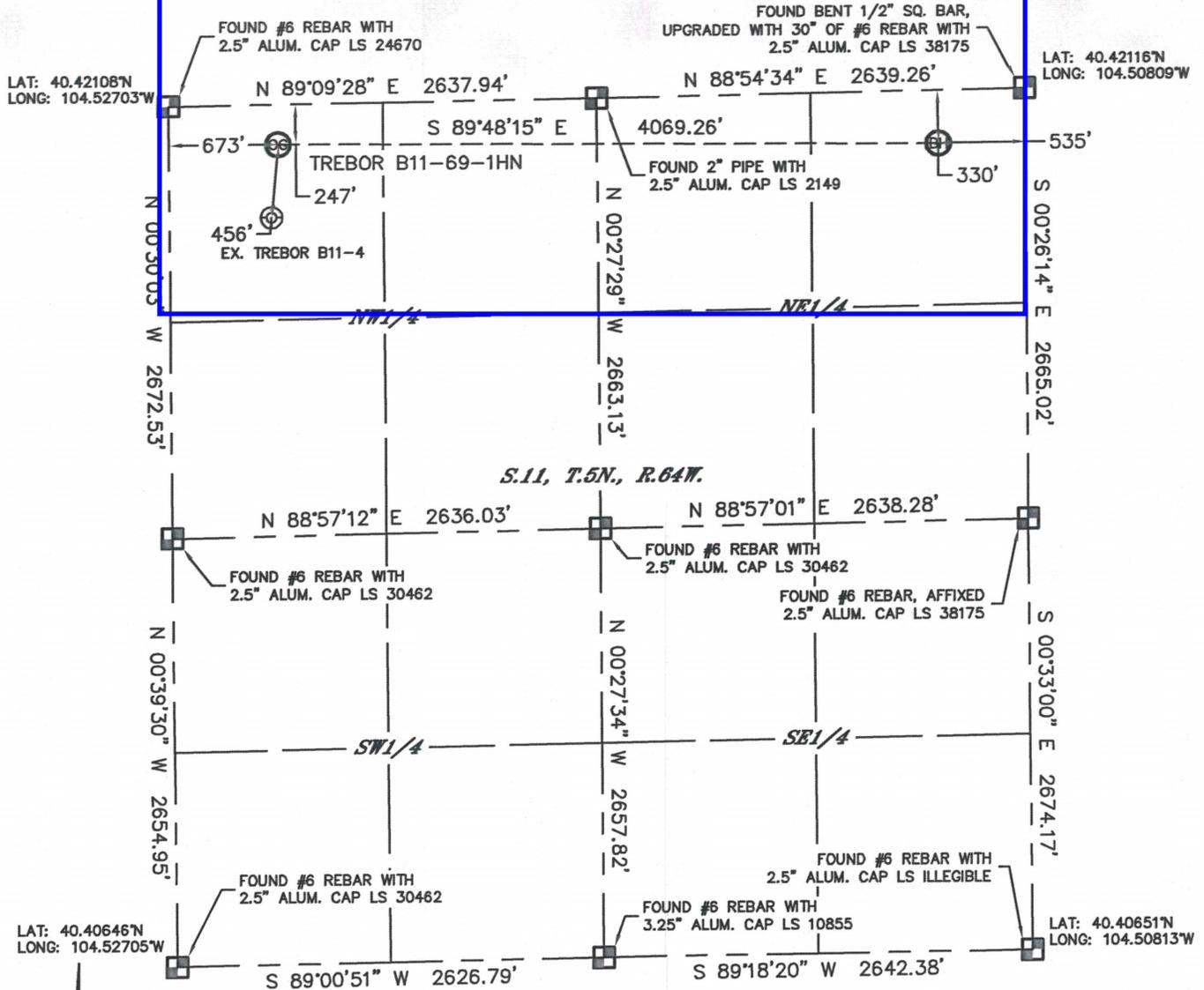
In accordance with a request from Mike Rodine with Noble Energy Inc., Lat40, Inc. has determined the surface location of the TREBOR B11-69-1HN to be 247' from the NORTH line and 673' from the WEST line and the bottom hole to be 330' from the NORTH line and 535' from the EAST line as measured at right angles from the section lines of Section 11, Township 5 North, Range 64 West of the Sixth Principal Meridian, County of Weld, State of Colorado.
