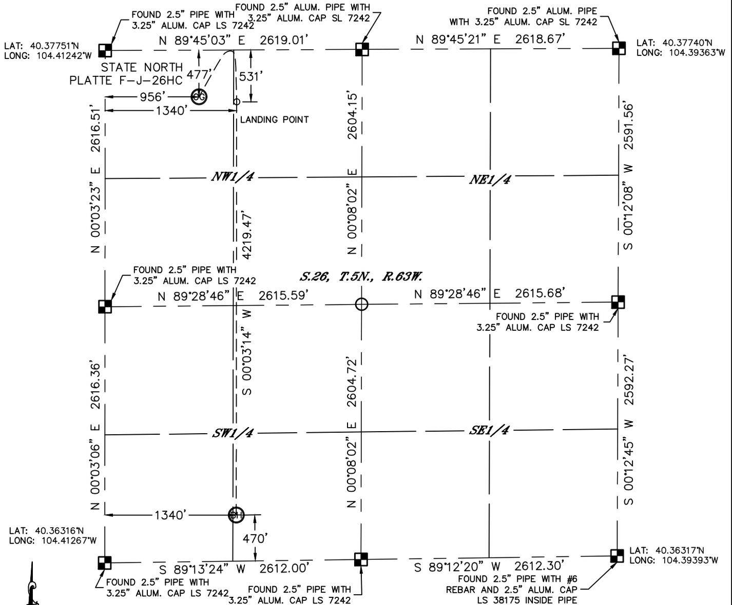
In accordance with a request from Michael Meagher with BONANZA CREEK ENERGY, INC. Lat40°, Inc. has determined the surface location of the STATE NORTH PLATTE F-J-26HC to be 477' from the NORTH line and 956' from the WEST line and the bottom hole to be 470' from the SOUTH line and 1340' from the WEST line as measured at right angles from the section lines of Section 26, Township 5 North, Range 63 West of the Sixth Principal Meridian, County of Weld, State of Colorado.
