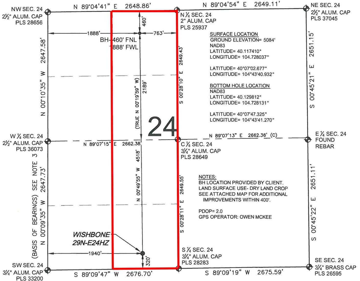
WELL WISHBONE 29N-E24HZ TO BE LOCATED 320' FSL AND 1940' FWL
