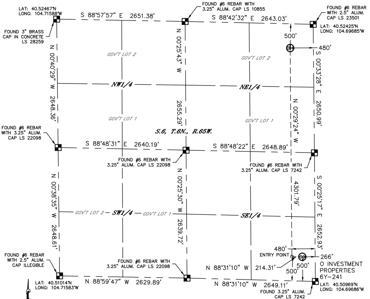
In accordance with a request from Jeff Dillingham with PDC ENERGY Lat40°, Inc. has determined the surface location of the O INVESTMENT PROPERTIES 6Y-241 to be 500' from the SOUTH line and 266' from the EAST line and the bottom hole to be 500' from the NORTH line and 480' from the EAST line as measured at right angles from the section lines of Section 6, Township 6 North, Range 65 West of the Sixth Principal Meridian, County of Weld, State of Colorado.
