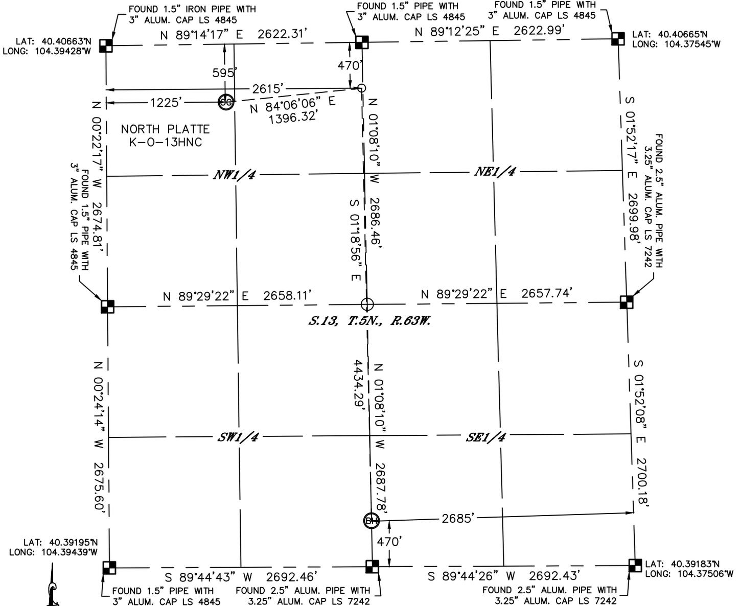
In accordance with a request from Keith Caplan with BONANZA CREEK ENERGY, INC. Lat40°, Inc. has determined the surface location of the NORTH PLATTE K-O-13HNC to be 595' from the NORTH line and 1225' from the WEST line and the bottom hole to be 470' from the SOUTH line and 2685' from the WEST line as measured at right angles from the section lines of Section 13, Township 5 North, Range 63 West of the Sixth Principal Meridian, County of Weld, State of Colorado.
