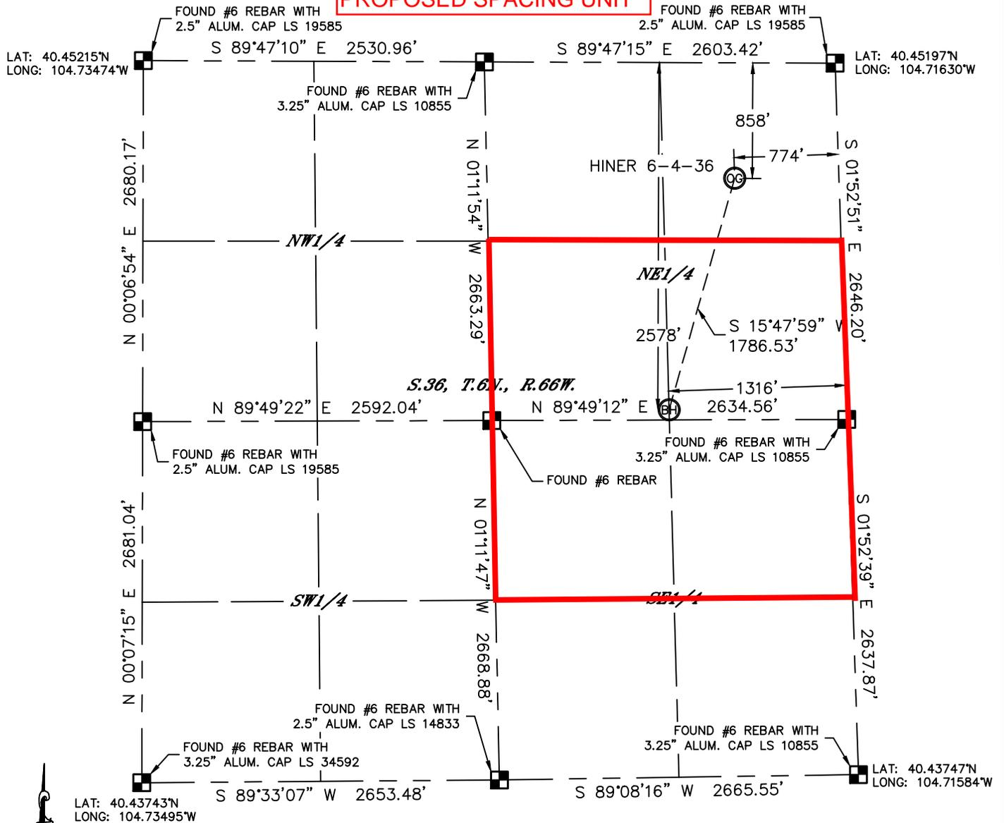
In accordance with a request from Clayton Duke with HRM RESOURCES, LLC Lat40°, Inc. has determined the surface location of the HINER 6-4-36 to be 858' from the NORTH line and 774' from the EAST line and the bottom hole to be 2578' from the NORTH line and 1316' from the EAST line as measured at right angles from the section lines of Section 36, Township 6 North, Range 66 West of the Sixth Principal Meridian, County of Weld, State of Colorado.
