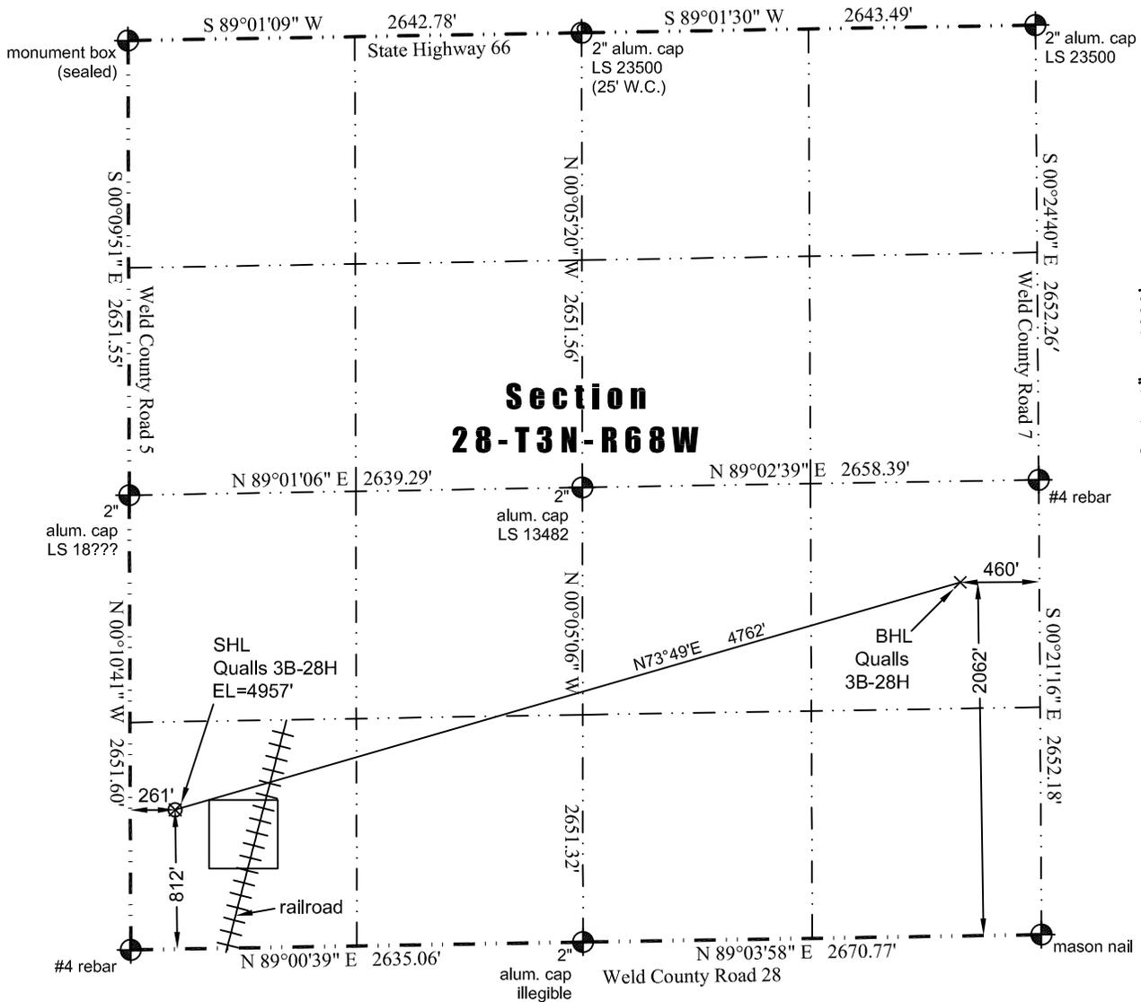
In accordance with a request from Jay Knutson of EnCana Oil & Gas (USA) Inc., JR Land Surveying, LLC has determined the location of the **Qualls 3B-28H** well site to be SHL: 812' FSL and 261' FWL, (BHL: 2062' FSL and 460' FEL), as measured at ninety (90) degrees from the section lines of Sections 28, Township 3 North, Range 68 West of the 6th Principal Meridian, Weld County Colorado.
