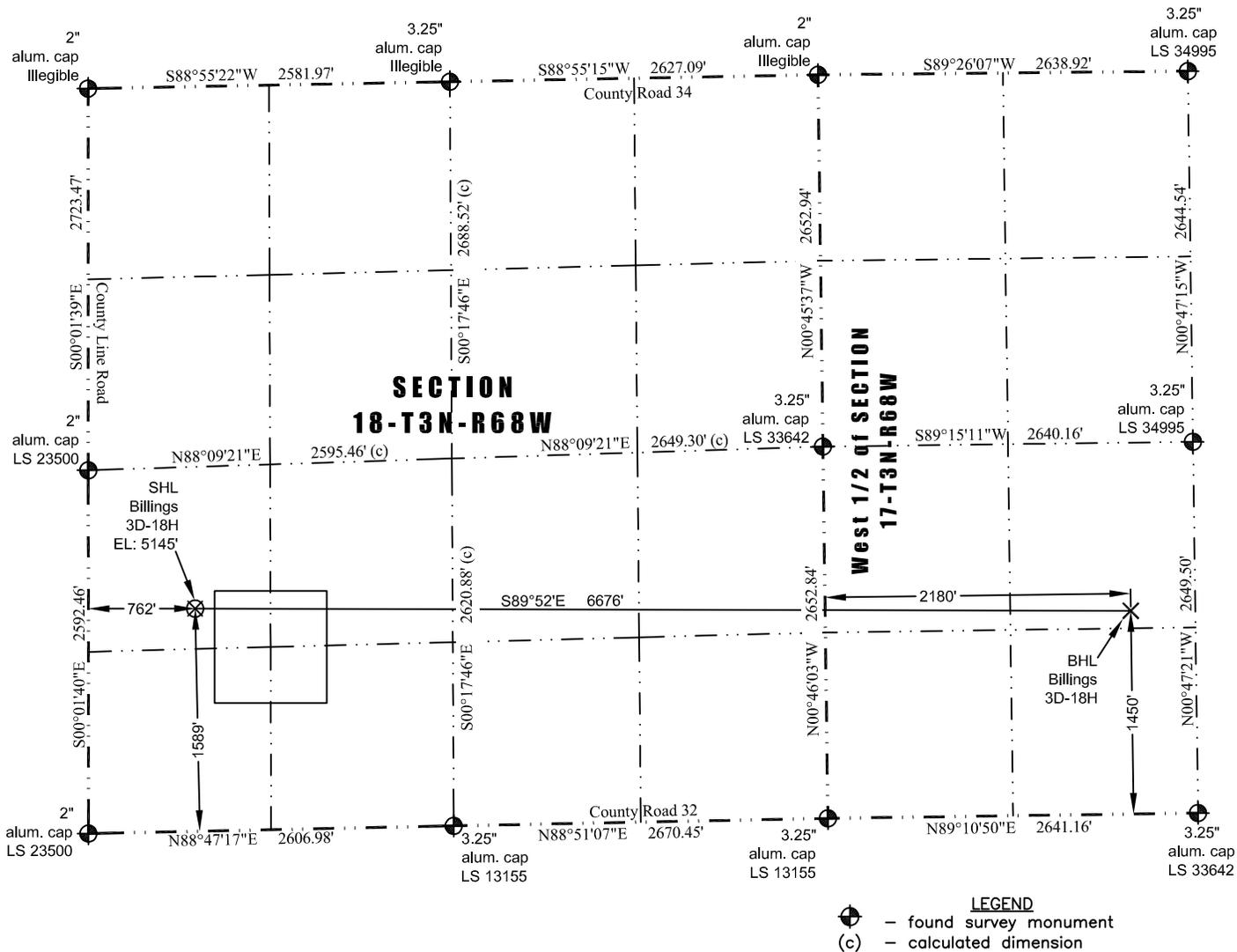
In accordance with a request from Jay Knutson of EnCana Oil & Gas (USA) Inc., JR Land Surveying, LLC has determined the location of the **Billings 3D-18H** well site to be SHL: 1589' FSL and 762' FWL, (BHL: 1450' FSL and 2180' FWL) as measured at ninety (90) degrees from the section lines of Section 18 and Section 17, Township 3 North, Range 68 West, 6th Principal Meridian, County of Weld, CO.
