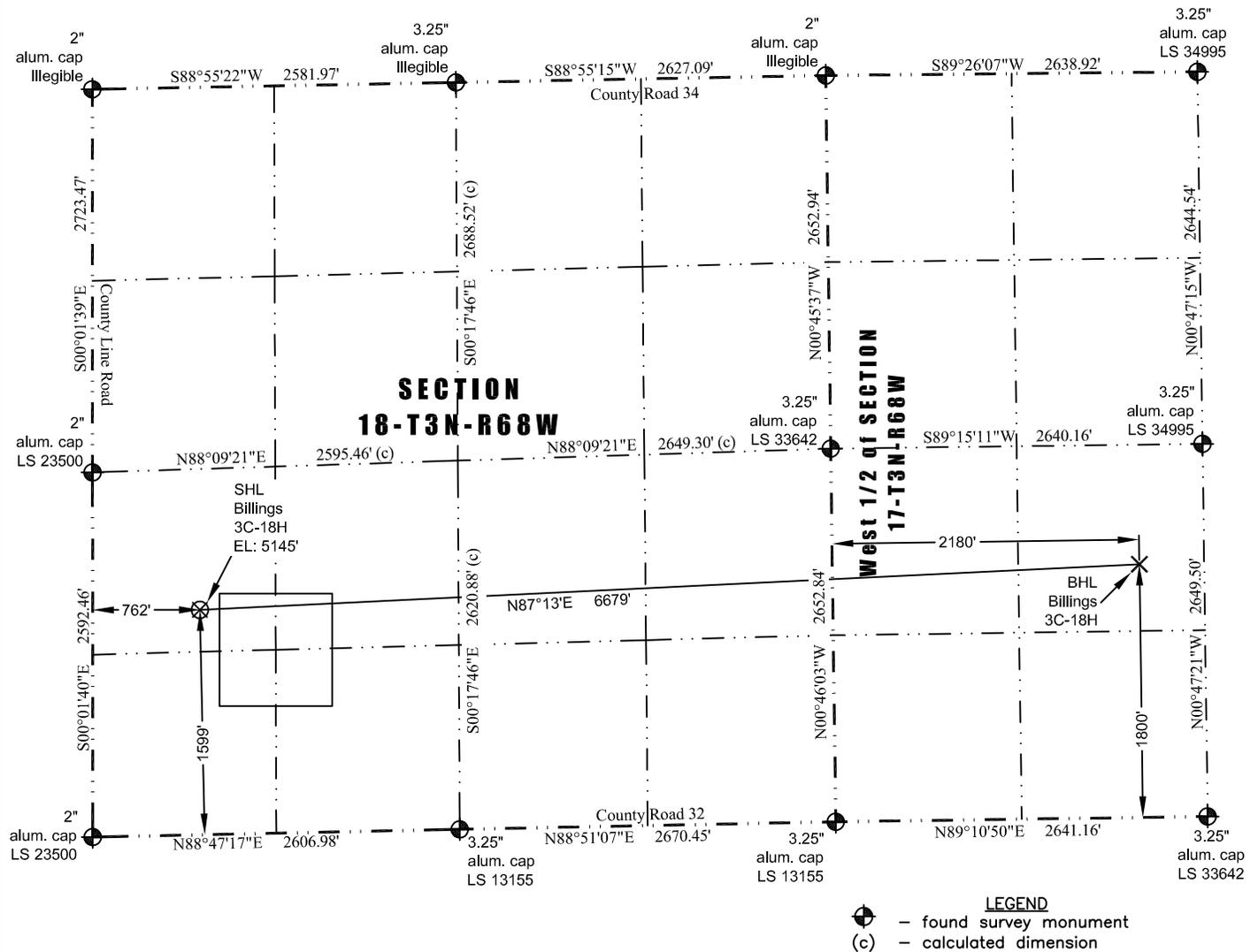
In accordance with a request from Jay Knutson of EnCana Oil & Gas (USA) Inc., JR Land Surveying, LLC has determined the location of the **Billings 3C-18H well** site to be SHL: 1599' FSL and 762' FWL, (BHL: 1800' FSL and 2180' FWL) as measured at ninety (90) degrees from the section lines of Section 18 and Section 17, Township 3 North, Range 68 West, 6th Principal Meridian, County of Weld, CO.
