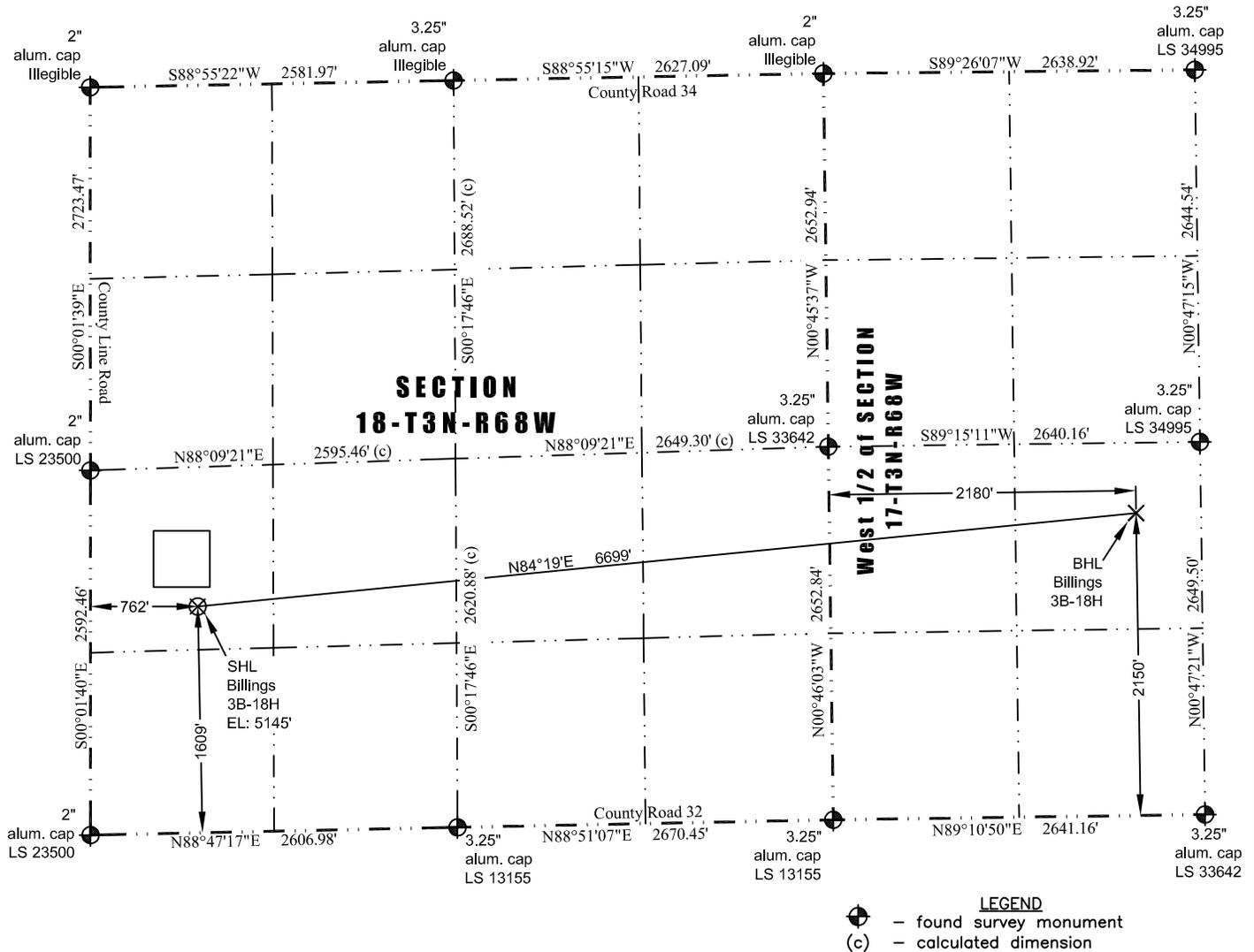
In accordance with a request from Jay Knutson of EnCana Oil & Gas (USA) Inc., JR Land Surveying, LLC has determined the location of the **Billings 3B-18H** well site to be SHL: 1609' FSL and 762' FWL, (BHL: 2150' FSL and 2180' FWL) as measured at ninety (90) degrees from the section lines of Section 18 and Section 17, Township 3 North, Range 68 West, 6th Principal Meridian, County of Weld, CO.
