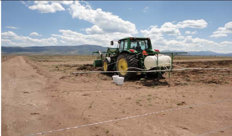
**Subject:** The concentrated Earth Smart hydrocarbon cleaner was delivered in 5-gallon containers. The area was treated twice using a ratio of one 5-gallon bucket of the concentrate to approximately 100 gallons of water.
