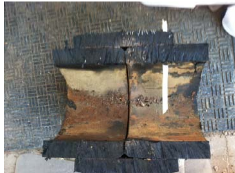
Fig 3 1/8" Gap on Top
