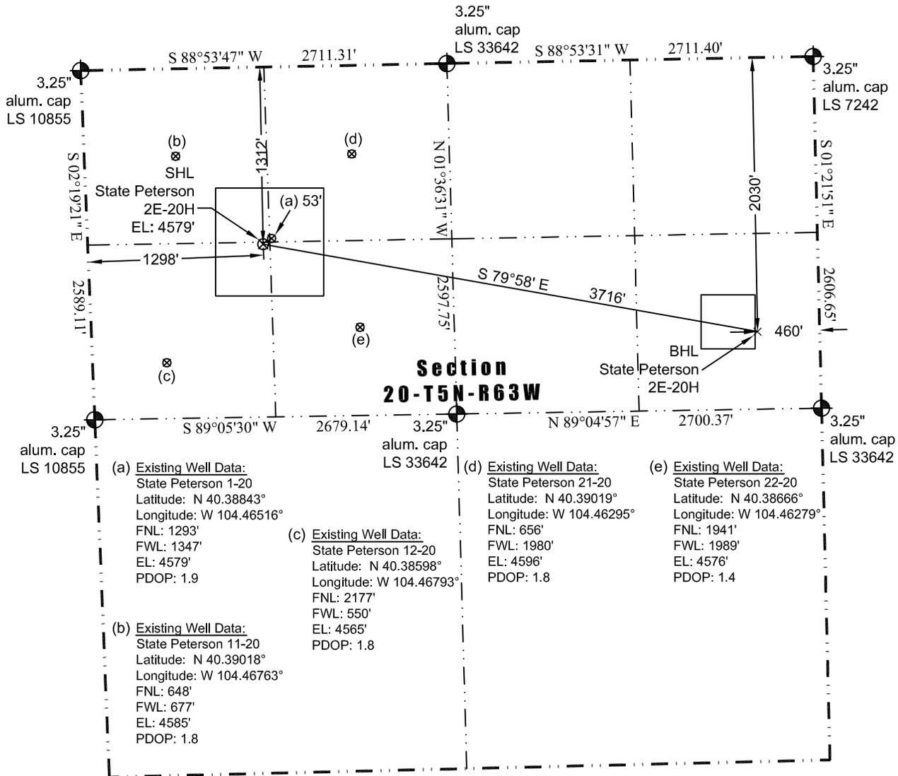
In accordance with a request from Jay Knutson of EnCana Oil & Gas (USA) Inc., JR Land Surveying, LLC has determined the location of the **State Peterson 2E-20H** well site to be SHL: 1312' FNL and 1298' FWL, (BHL: 2030' FNL and 460' FEL) as measured at ninety (90) degrees from the section lines of Section 20, Township 5 North, Range 63 West, 6th Principal Meridian, Weld County, CO.
