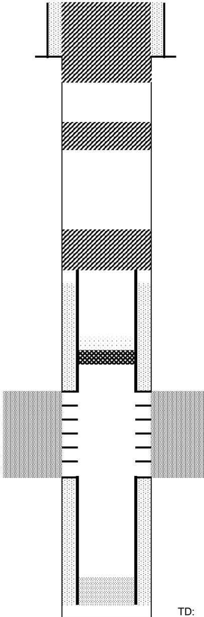
Cut surface casing off 6'-8' below surface.
