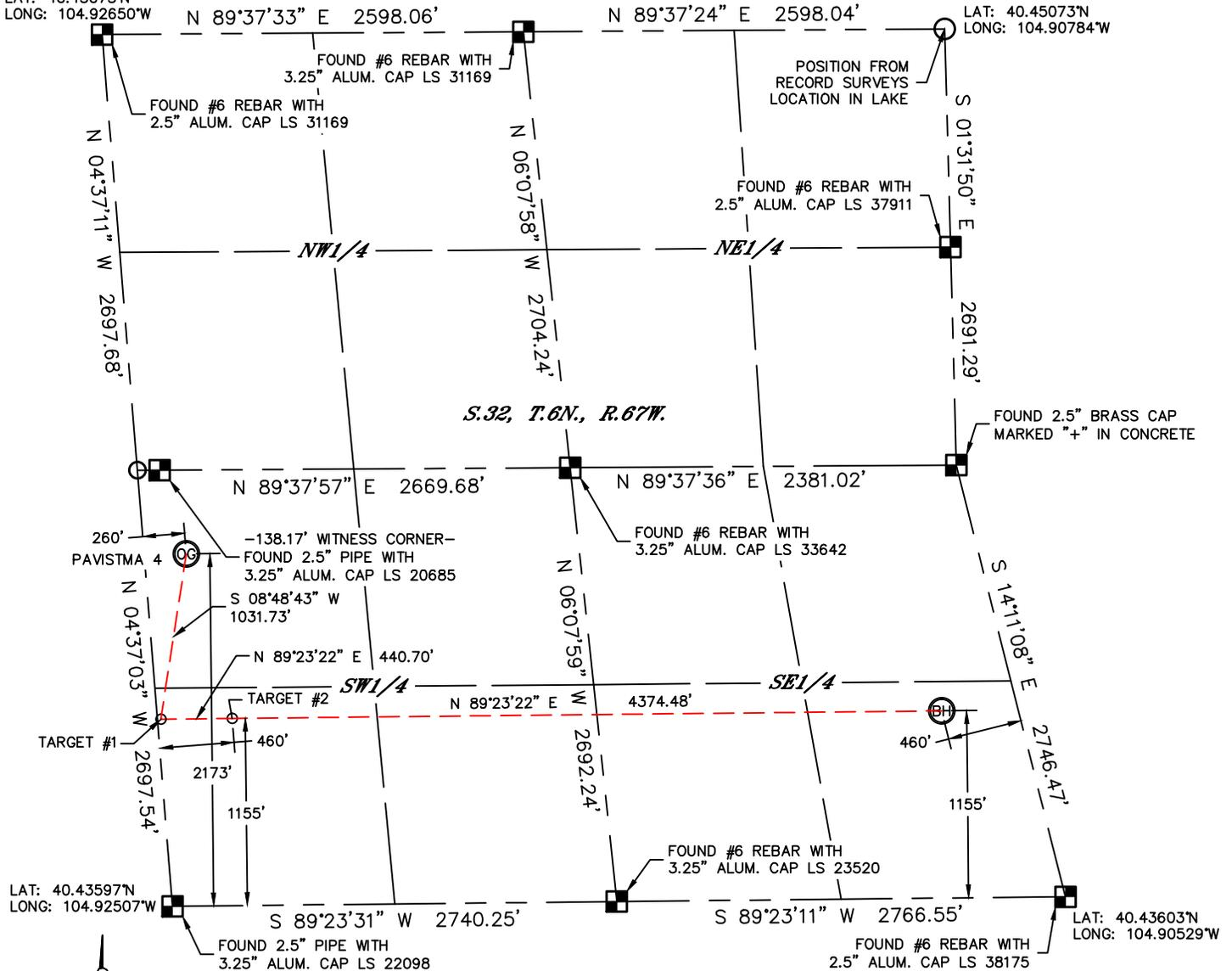
In accordance with a request from Michael Cuba with TEKTON ENERGY, LLC Lat40°, Inc. has determined the surface location of the PAVISTMA 4 #1-6-32-090-4-NH to be 2173' from the SOUTH line and 260' from the WEST line and the bottom hole to be 1155' from the SOUTH line and 460' from the EAST line as measured at right angles from the section lines of Section 32, Township 6 North, Range 67 West of the Sixth Principal Meridian, County of Weld, State of Colorado.
