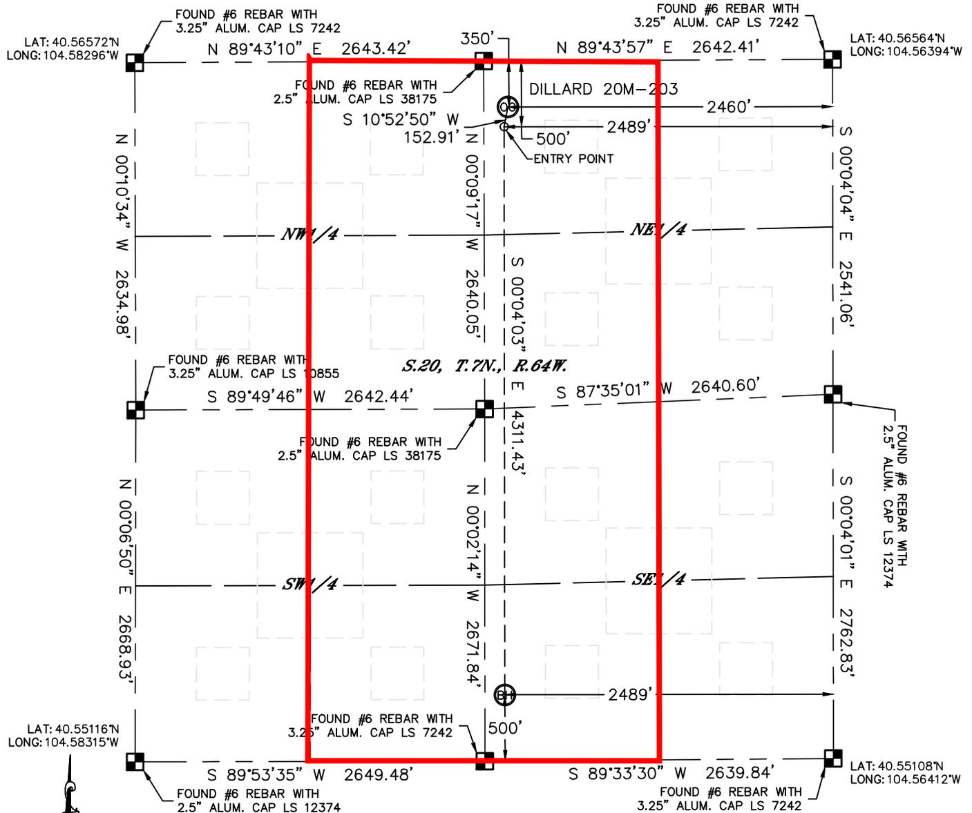
In accordance with a request from Al Bragg with PDC Energy Lat40°, Inc. has determined the surface location of the DILLARD 20M-203 to be 350' from the NORTH line and 2460' from the EAST line and the bottom hole to be 500' from the SOUTH line and 2489' from the EAST line as measured at right angles from the section lines of Section 20, Township 7 North, Range 64 West of the Sixth Principal Meridian, County of Weld, State of Colorado.
