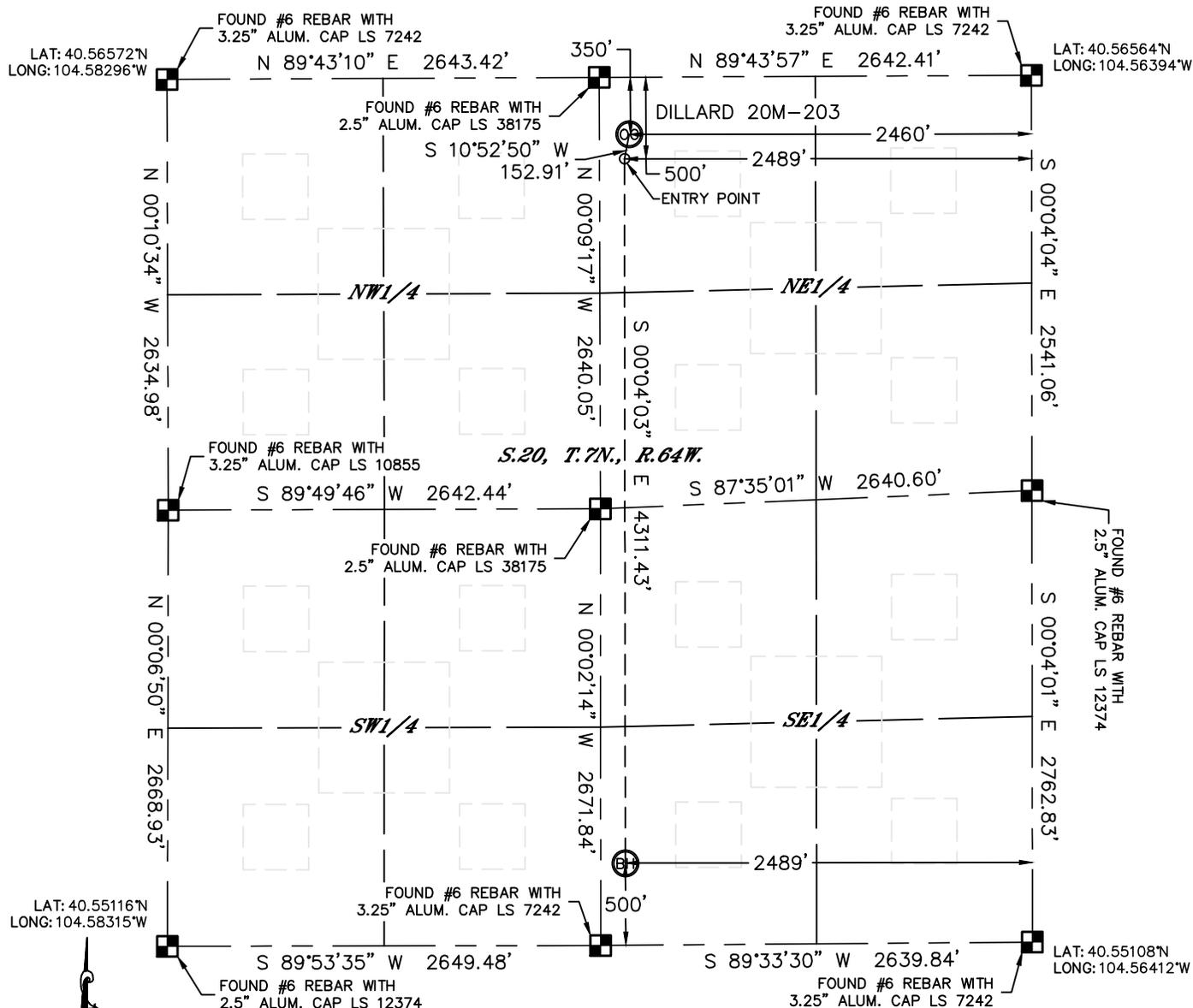
In accordance with a request from Al Bragg with PDC Energy Lat40°, Inc. has determined the surface location of the DILLARD 20M-203 to be 350' from the NORTH line and 2460' from the EAST line and the bottom hole to be 500' from the SOUTH line and 2489' from the EAST line as measured at right angles from the section lines of Section 20, Township 7 North, Range 64 West of the Sixth Principal Meridian, County of Weld, State of Colorado.
