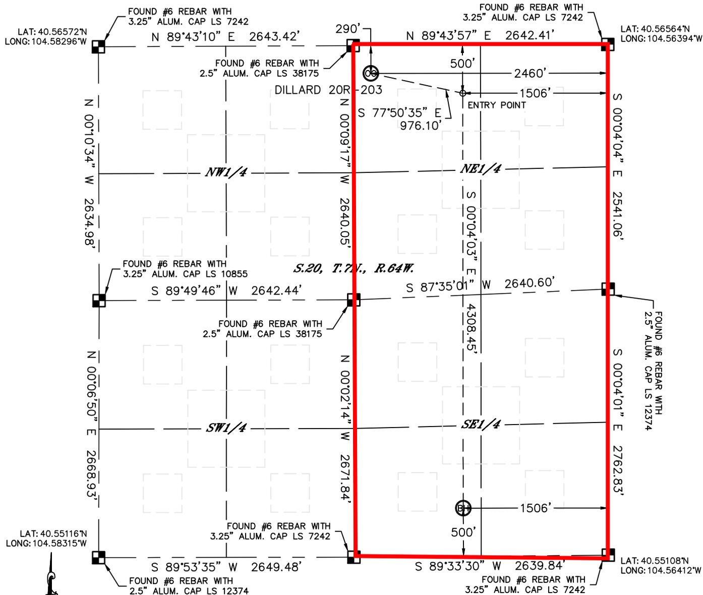
In accordance with a request from Al Bragg with PDC Energy Lat40°, Inc. has determined the surface location of the DILLARD 20R-203 to be 290' from the NORTH line and 2460' from the EAST line and the bottom hole to be 500' from the SOUTH line and 1506' from the EAST line as measured at right angles from the section lines of Section 20, Township 7 North, Range 64 West of the Sixth Principal Meridian, County of Weld, State of Colorado.
