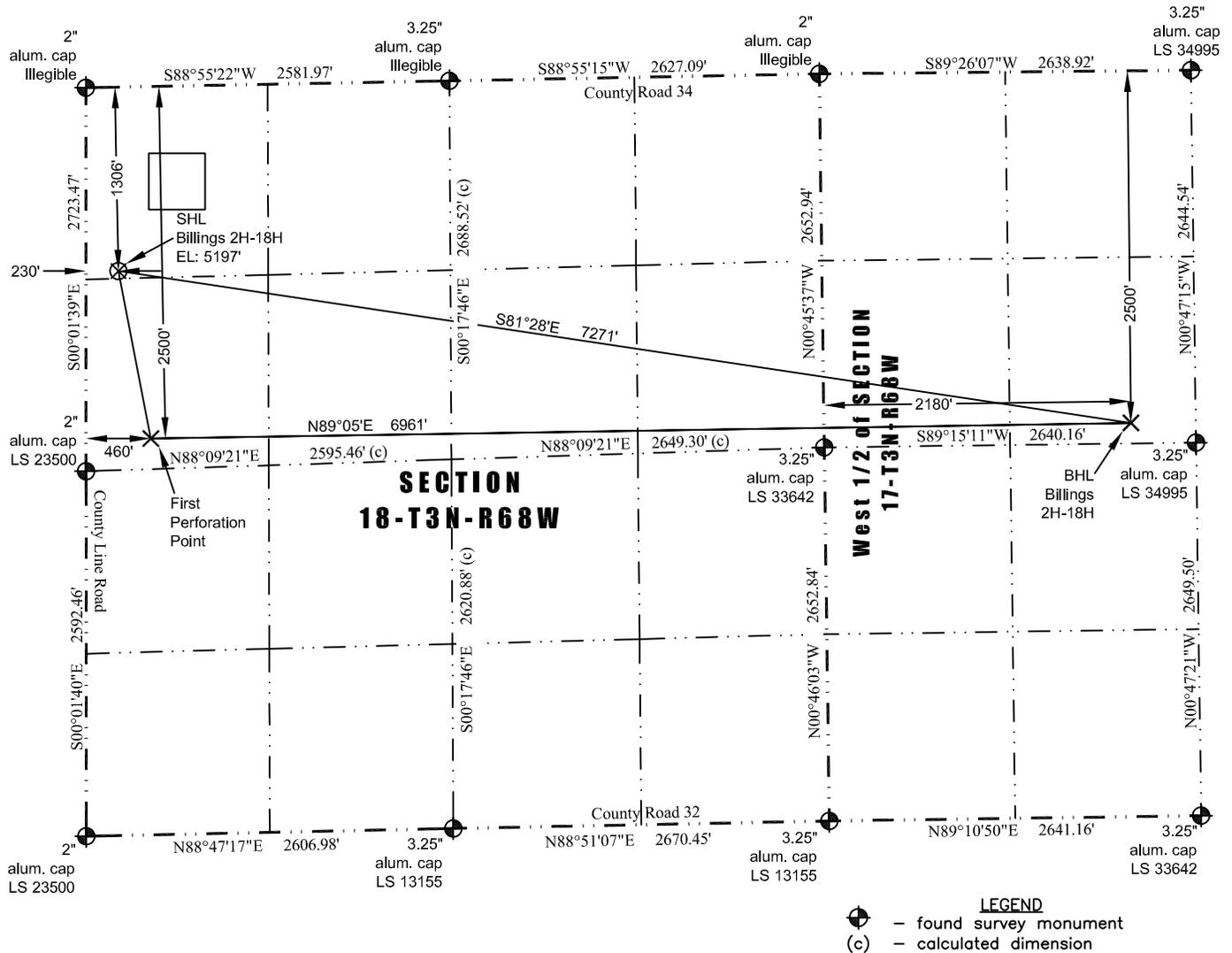
In accordance with a request from Jay Knutson of EnCana Oil & Gas (USA) Inc., JR Land Surveying, LLC has determined the location of the **Billings 2H-18H** well site to be SHL: 1306' FNL and 230' FWL, (BHL: 2500' FNL and 2180' FWL) and (First Perforation Point: 2500' FNL and 460' FWL) as measured at ninety (90) degrees from the section lines of Section 18 and Section 17, Township 3 North, Range 68 West, 6th Principal Meridian, County of Weld, CO.
