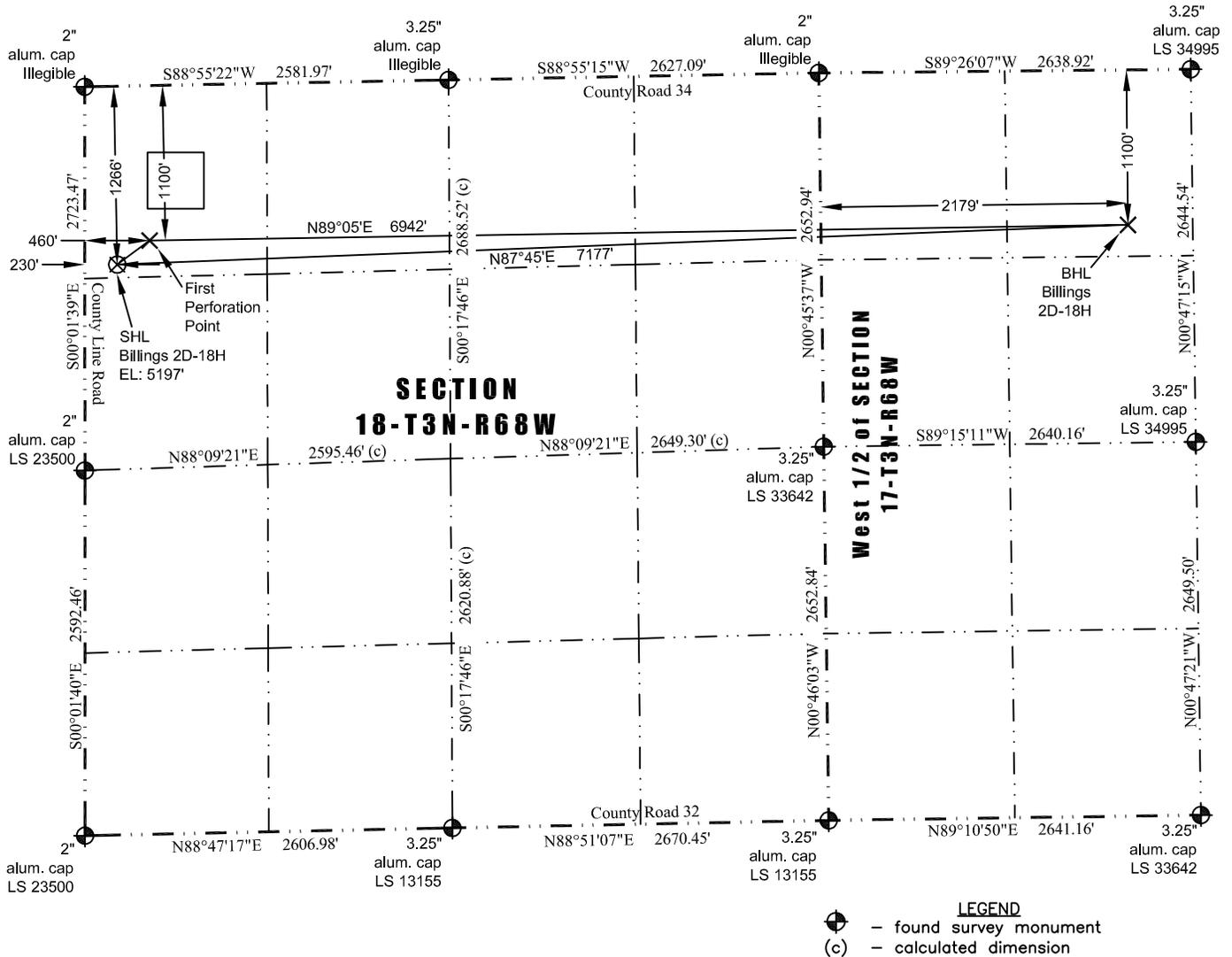
In accordance with a request from Jay Knutson of EnCana Oil & Gas (USA) Inc., JR Land Surveying, LLC has determined the location of the **Billings 2D-18H** well site to be SHL: 1266' FNL and 230' FWL, (BHL: 1100' FNL and 2179' FWL) and (First Perforation Point: 1100' FNL and 460' FWL) as measured at ninety (90) degrees from the section lines of Section 18 and Section 17, Township 3 North, Range 68 West, 6th Principal Meridian, County of Weld, CO.
