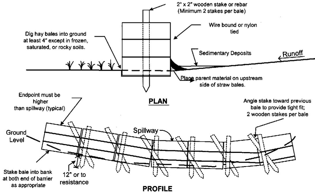
**3.3.1.3 Slope Breaker Construction & Placement**
