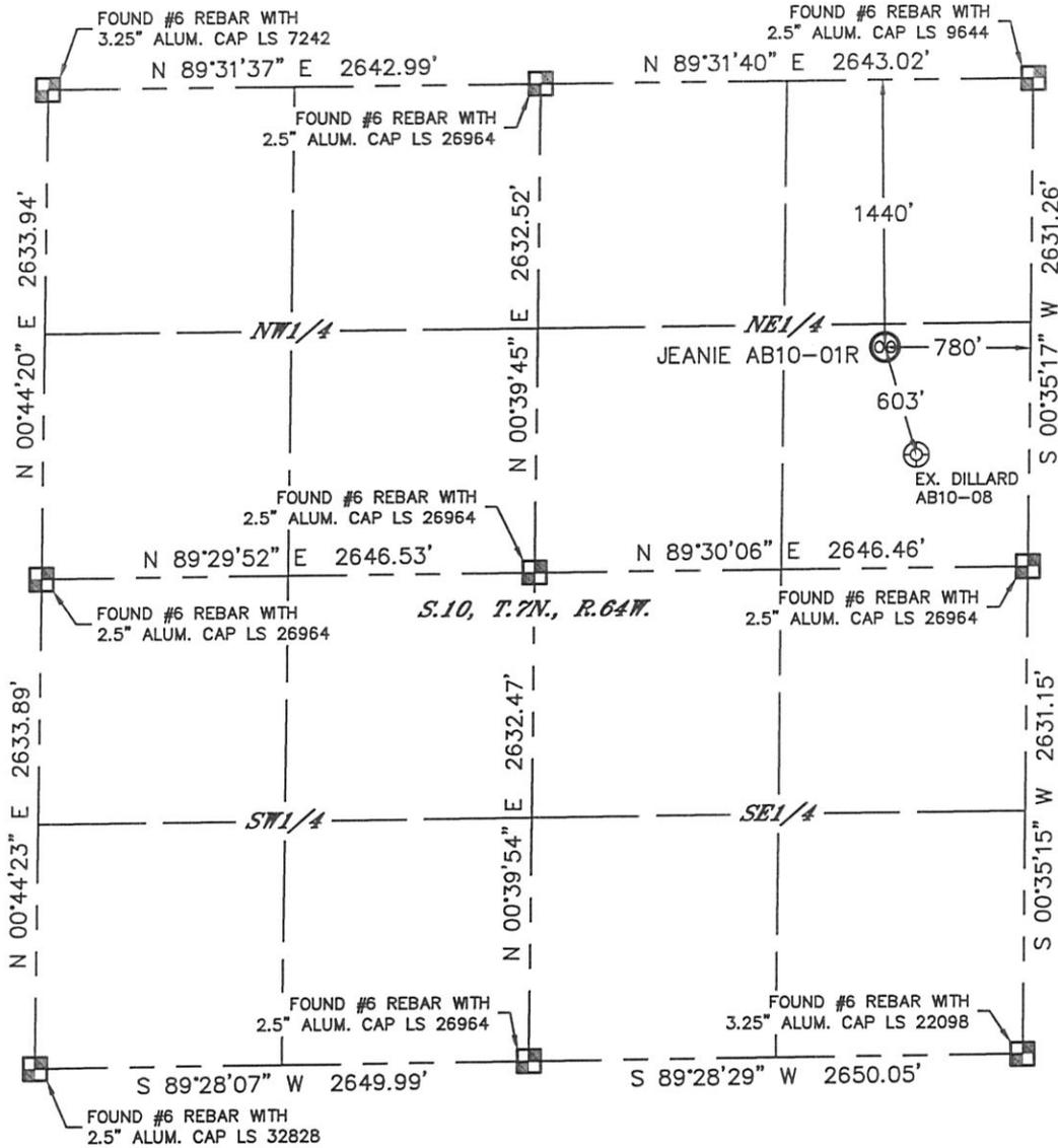
In accordance with a request from Jim Curry with Noble Energy Inc. Lat40°, Inc. has determined the surface location of the JEANIE AB10-01R to be 1440' from the NORTH line and 780' from the EAST line as measured at right angles from the section lines of Section 10, Township 7 North, Range 64 West of the Sixth Principal Meridian, County of Weld, State of Colorado.
