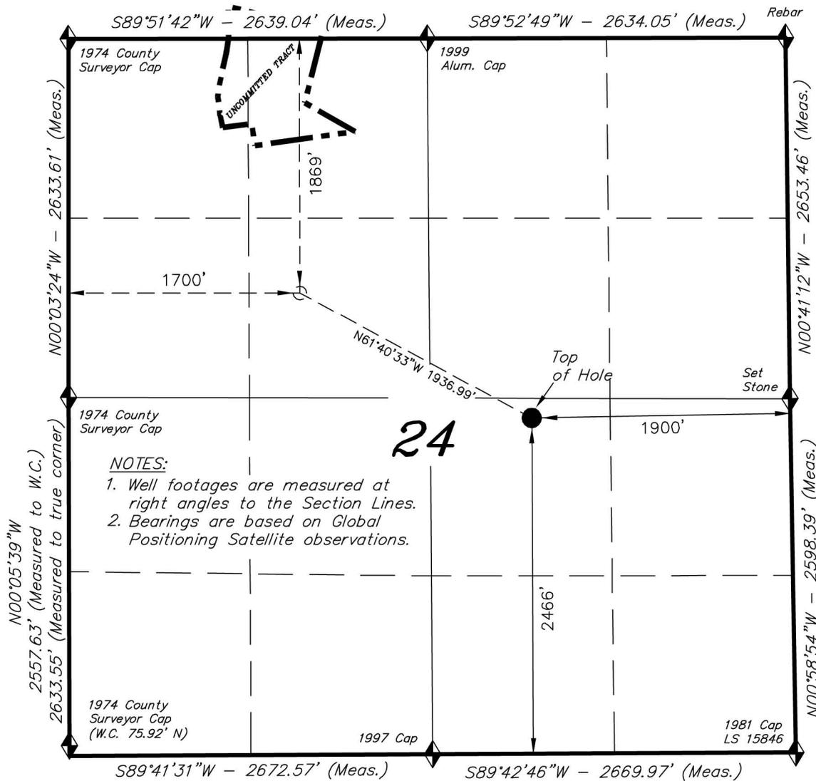
WELL LOCATION, ALP FEE 24-6B (J24), LOCATED AS SHOWN IN THE NW 1/4 SE 1/4 OF SECTION 24, T6S, R93W, 6th P.M. GARFIELD COUNTY, COLORADO.
