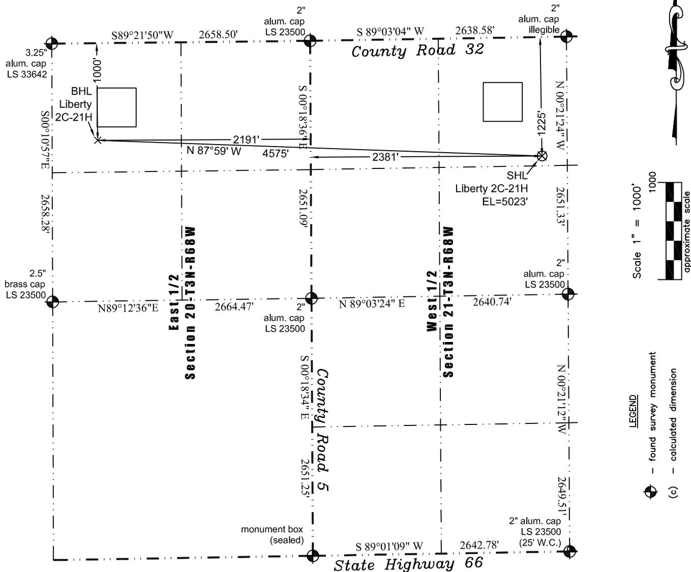
In accordance with a request from Jay Knutson of EnCana Oil & Gas (USA) Inc., JR Land Surveying, LLC has determined the location of the **Liberty 2C-21H** well site to be SHL 1225' FNL and 2381' FWL (BHL 1000' FNL and 2191' FEL) as measured at ninety (90) degrees from the section lines of Section 20 and Section 21, Township 3 North, Range 68 West of the 6th Principal Meridian, Weld County, Colorado.
