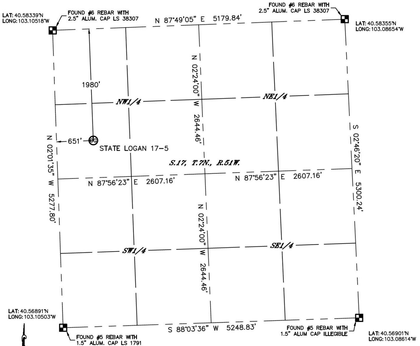
In accordance with a request from Robert Anderson with Overland Resources, LLC Lat40°, Inc. has determined the surface location of the STATE LOGAN 17-5 to be 1980' from the NORTH line and 651' from the WEST line as measured at right angles from the section lines of Section 17, Township 7 North, Range 51 West of the Sixth Principal Meridian, County of Logan, State of Colorado.
