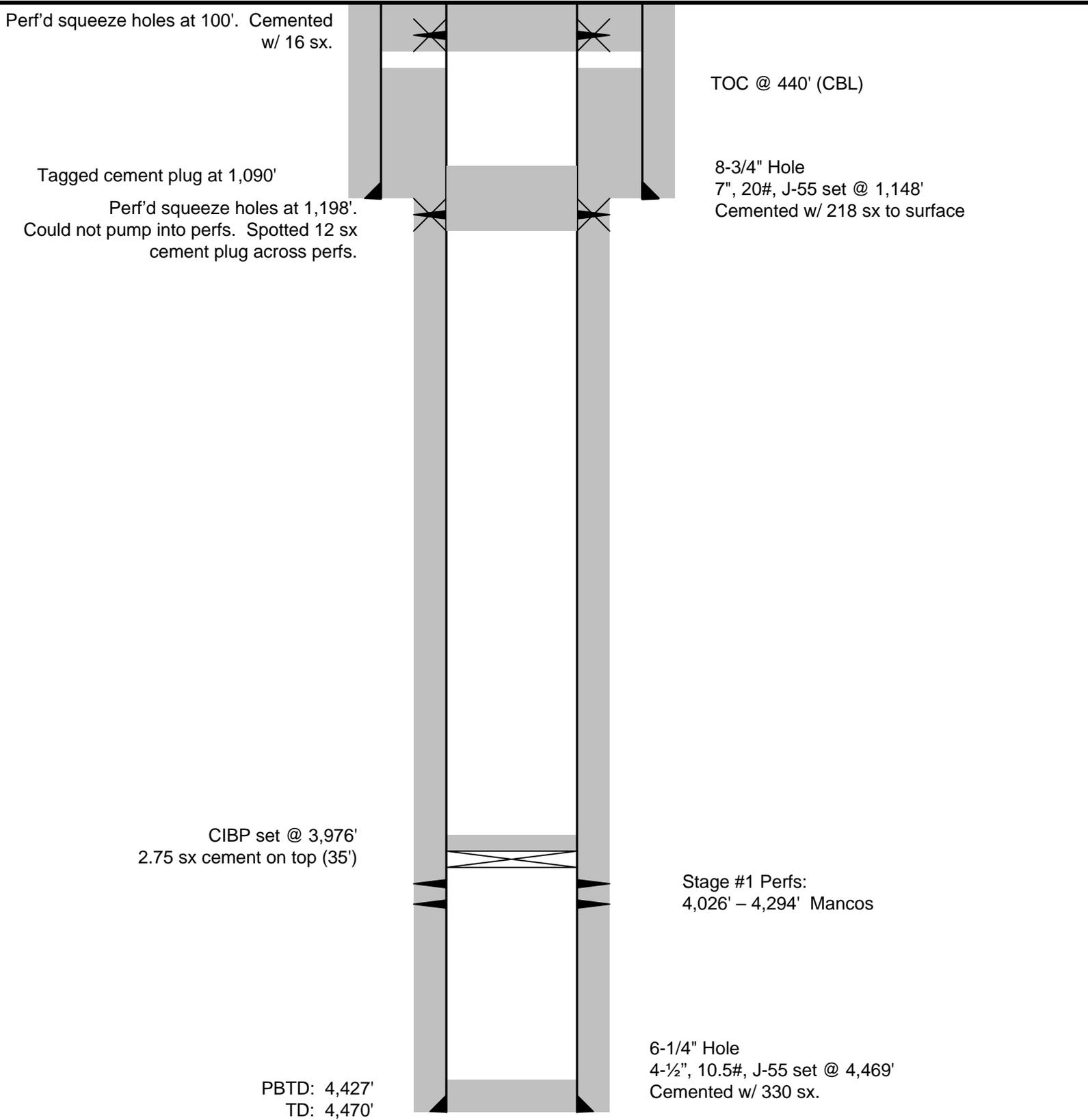
Perf'd squeeze holes at 100'. Cemented w/ 16 sx.
